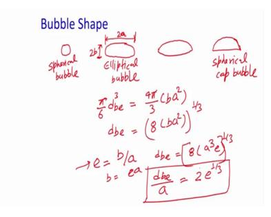
So, generally the bubble 4 type of bubble shape is being reported in the literature and, the first shape is if the bubble is very small in diameter it will be cynical in nature. So, you will see a very pretty much spherical bubble. So, if the bubble is small you will see the spherical size bubble, but if you put more gas then what will happen before detachment bubble size will increase.
