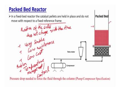
If you talk about the with the time the particle movement will be 0 they will not be moving so that this kind of a bed where the particle is being dumped, or catalysts are being dumped and, they held at a certain place and their place or their position does not change with the time it is called as a packed bed. So, the position of the solid they move certain things, but not much position of the solid they can vibrate, but they cannot move solid change with the time.
