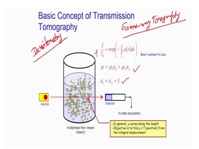
Then we move to the ionizing system and the ionizing system based on that gamma ray densitometry that works on the transmission tomography principle. So, what we are going to discuss is the gamma ray tomography or X-ray tomography. Now the gamma ray based principle of the gamma ray tomography is relatively simpler; what we do here is we take a source, we take a detector just the detector is similar to as of use in the RPT technique.
