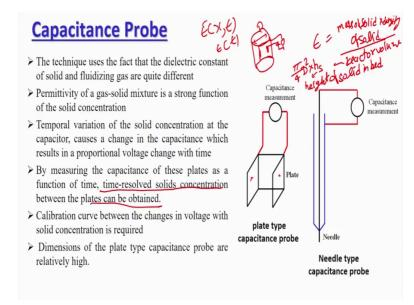
So, now start with the capacitance probe what happen in the capacitance probe; we use the permittivity of different material we know that the permittivity of different material is different and we use that principle to calculate the volume fraction. So, what we do here we take two plates; this two plates we take and between these two plates we give certain voltage.
