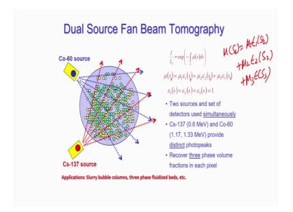
So, this if you want to have three phase bed suppose if you want to have a three phase fluidized bed or you have a slurry bubble column. And you want to measure the volume fraction by using the tomography what you can do instead of the single beam tomography you can have dwell beam tomography.
