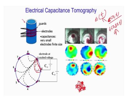
So, how it works? As I said you have suppose this is the system, you put the electrodes all around the periphery on the periphery of the system all around it. Now suppose you have 8 probe system, you have 8, you have taken 8 probe what we do we slowly start exciting the probes ok.
