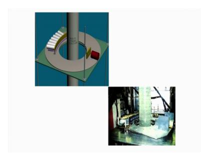
Now, if you want to have a pixel wise information or detailed information of the volume fraction distributed on the pixel wise; what we need to do? We need to acquire the data in a different way. So, how we can acquire the data? We can have two kind of a projection; one case we can use one detector one source several detectors and in other case we can use several source and several detectors.
