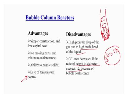
The major advantage of the bubble column is that as a very simple construction. As I said that is just a column you have to take you have to put a distributor or sparger which can distribute the air inside the liquid, if it is in the batch it makes your system further simpler you do not need any pump; you have to just dump the liquid inside you pass the gas.
