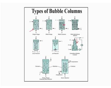
So, what we are going to see that; this based on this regime actually and based on that operation that I said that the major problem comes in to churn turbulent regime, because you have wide bubble size distribution lot of different bubble type columns is being introduced where different types of the bubble column is being introduced to come over that bigger bubble size distribution problems.
