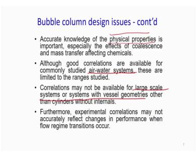
So, these are the design parameter which one require to understand the bubble the another design parameter which is required to understand or to have the knowledge is about the physical property. So, what is the liquid; and gas we are using what is the property of it; and this physical property is very important to determine the coalescence and the mass transfer.
