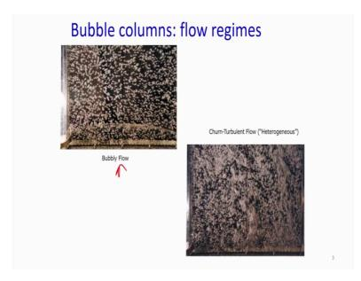
Now, there is different flow regimes occur in the bubble column the main two main regime which is being used at the industrial label is bubbly flow in the bubbly flow you can see the photograph this is a typical photograph of the bubbly flow the small tiny bubbles are formed.
