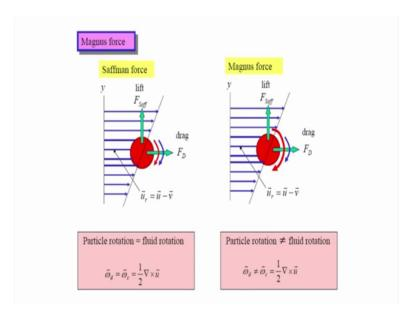
So, similar way Magnus force is also being defined and the Magnus force is being defined because of the particle friction. So, if there is a frictional difference is there between the same particle then the force which will be act is called the Magnus force, the if this the pressure radiant then it is called the lift force.
