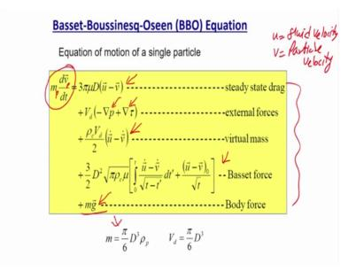
So, that is what is the Basset history force virtual mask force. So, finally, if I write the forces which is acting across one particle which is given by the Basset Boussinesq Oseen equation which is famously known as BBO equation, which we have done earlier also we can write that at steady state for one particle not a steady state sorry, in the motion equation of motion for a single particle should be given in this form.
