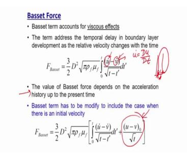
Because of the viscosity of a some force act on the body and that force is called the Basset force ok. This force actually also act the temporal delay in the boundary layer development as the relative velocity changes with the time.
