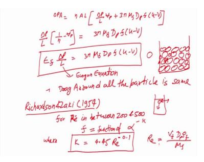
So, I can write it delta P upon A is equal to nothing, but number density into area into L into delta P upon L, volume of a single particle plus 3 pi mu of fluid, D of particle f into u minus v this way we can write it.
