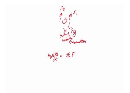
But different other forces also act on the particle, some forces are important for the gas liquid application, some forces are important for the gas solid applications, but there are other forces also which affect the motion of the discrete phase. Now again I am saying discrete phase because it can be droplet, it can be bubble, it can be particle. So, other forces also act and we need to define now those other forces and those other forces are
