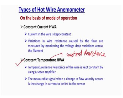
Now, based on the mode of operation, how you want to operate the hot wire anemometry is actually being divided mainly in 2 parts that, one is called constant current hot wire anemometer, and second one is called constant temperature hot wire anemometer. Now as the name suggests that in the constant current you are going to keep the currents same, and in the constant temperature you are going to keep the temperature same.
