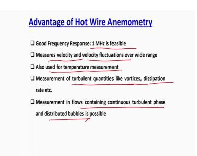
So, now concluding this part of hot wire anemometer, what I will say that advantage of the hot wire anemometer it has the major advantage there is a very good frequency response, it means the temporal response is very very high.
