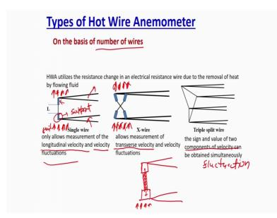
Now the types has been divided based on number of wires. And also based on the wave mode of operation. So, we discuss the wave mode of operation before that I will discuss that number of wires, that has been kind of divided the 1, first one is called single wire as I have discussed and the photograph I have already shown you, this is a single wire anemometer. So, what it does it does that the single wire anemometer is being placed in the flow ok.
