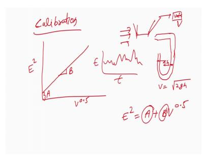
So, what we do we do the calibration, and in the calibration what we do in the calibration part, we suspend the probe in a domain say this is the fluid field or and I suspend the wire here, I suspend the wire. So, this is the probe I suspended it here, somewhere here in this way the prong, I suspend the wire and I measure that velocity. Now how I measure the velocity what I do I put a pitot tube, and that is the way the calibration is being done in hot wire anemometer.
