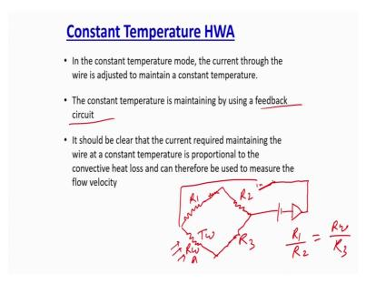
So, what is the constant temperature in constant temperature mode what we do, the current through the adjust wire is adjusted to maintain the constant temperature. So, how the temperature will be given, if I maintain that current constant then what will happen that sorry if you want to maintain the temperature constant, what you need to do you have to vary the current. So, suppose this is the Wheatstone bridge again I will make the same.
