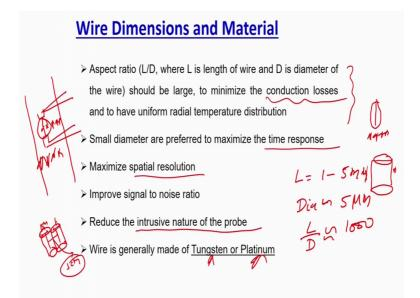
Now, this hot wire anemometer though we can buy from a commercial vendor, but ideally speaking you can also prepare the hot wire anemometer at your place, and is very simple to make you just need a wire made of tungsten or platinum. So, both of this kind of most of this wires used in the hot wire anemometer is either made of tungsten or made of platinum, some of sometimes they are mixed materials also.
