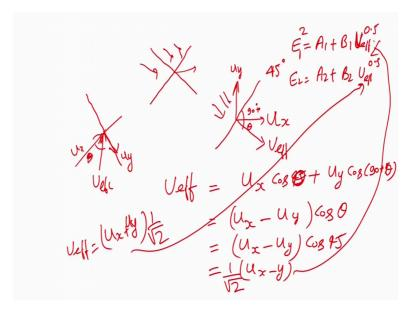
So, what you can do if suppose I use a x wire I will just so, 1 example triplet will be the same you can try to do that. So, suppose if I am using the at wire and there is a velocity in this direction. Let us do it with the 1 wire which is being inclined. Now this is say velocity, this is the you are going to get it in this way.
