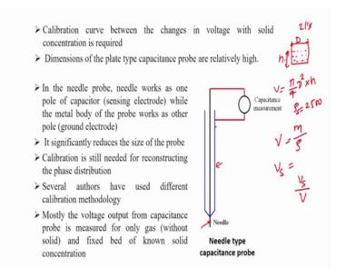
To overcome that a different type of capacitance probe has been developed and that is called needle type capacitance probe ok.
