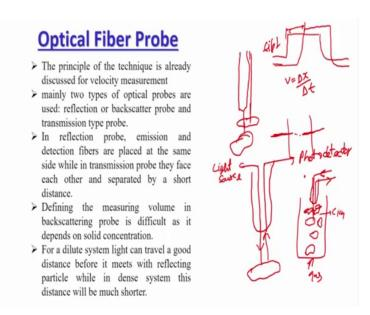
So, next is optical fiber probe; now we have already discussed the optical fiber probe in the velocity measurement technique, and the that time also I said that this technique can be used to measure the volume fraction I try to briefly explain it at that moment, but what we are going to discuss we are now going to see that how this technique will be used to measure the volume fraction.
