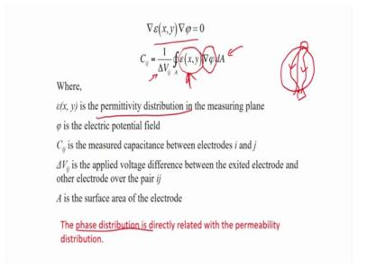
So, that permittivity distribution can be said as the phase distribution, its directly proportional. So, what you do? You measure the electric potential across the each probe how its there, and that electric potential is actually the related with the del epsilon into del phi will be equal to 0.
