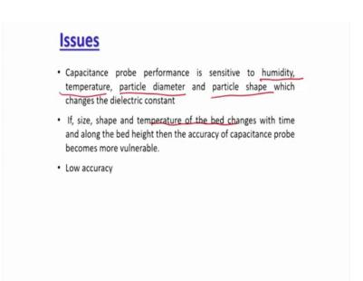
So, that is the way it has been measure. So, this is the technique is used and you see that if the technique and only other than the calibration part the technique is quite simple, it is very cheap you just need the two plates or one needle, which will be kind of grounded with the wall of the probe and you can measure the volume fraction.
