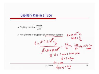
Now, let us just put the numbers here to have an idea about the capillary rise. So, a typical let us say we take a capillary of 10-micron diameter. So, the radius is 50 micron. oh sorry um 50 micron or 50 to 10 to minus 6 meters. So, h is equal to for water 2 into we again take cos theta is equal to half 2 into 7.2 into 10 to the power minus 2 is the surface transfer for air water cos theta.
