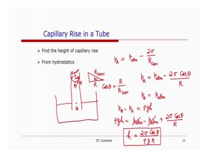
So,. So, we will look at the rise of capillarity from different angles and try to find the relationship. So, capillary rise in a liquid if we consider the capillary and consider a point b here and consider point just below it as point a. And the contact angle is theta. So, the pressure at point a is atmospheric pressure minus 2 sigma over radius of curvature of this interface. So, it is a cylindrical tube and this interface it has a a spherical shape, and it will be a part of a sphere.
