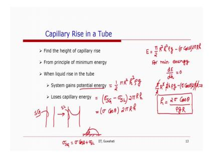
Now, you can also use the principle of energy minimization to obtain the height of capillary rise. So, when we have a liquid rising in a tube then there are 2 changes in the energy. The system gains some potential energy, which is equal to half pi R square h square rho g. And the system loses capillary energy which h equal to sigma SG.
