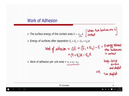
So, the surface energy of the contact area, after the contact the surface energy for the contact area is sigma 1 2 into a; that is the energy when 2 bodies are in contact. before contact or after this contact has been removed and the bodies are separate, the energy will be E 1 plus E 2. So, that is sigma 1 plus sigma 2 into A. So, sigma 1 and sigma 2 are the surface tensions of body 1 and body 2.
