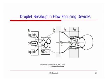
Now, for flow focusing devices; so, in the flow focusing device, a typical flow focusing device that had been taken by taken from article by the Garstecki et all. And the discussion we have is based around the article or the discussion in the article here.
