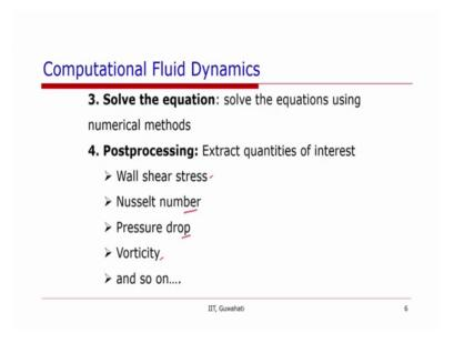
So, you have a number of algebraic equations, and then we need to use generally an iterative solver to solve these equations. And once we solve the equation, what we will get? We will get the values of the 3 velocity components, or the 2 velocity components depending on 2D or 3D problem and the pressure.
