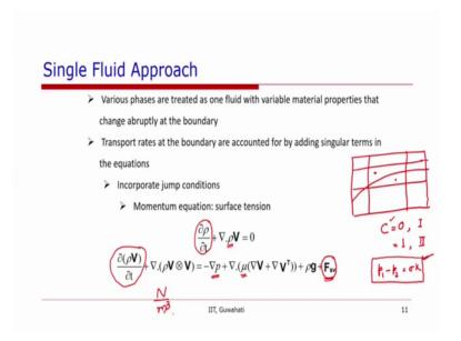
So, in the single fluid approach, we treat that all the phases are one material. Now if you look at these equations, in this we have 2 properties. One is density, and another is viscosity of the 2 fluids. So, one need to identify, when we have an interface and it this interface is to be captured than in such case, we will have at any point in a space, except at the interface; one will have that the fluid is either fluid 1 or fluid 2.
