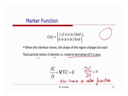
So, let us look at the marker function, marker function is that it has one value one in one fluid and 0 in another fluid. And when this interface moves; so, when the interface moves, the shape of the region changes, but each fluid particle has it is identity so; that means, this material derivative is 0. So, that is why we have del C over del t plus v dot del C or DC by DT is equal to 0.
