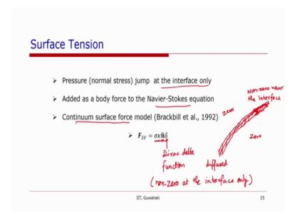
Having clarified that marker function or that we need to solve one equation for the marker function, and how do we find the curvature of the interface. Let us look at how we can include the surface tension.
