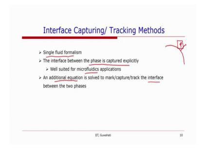
So, for the 2 phase flows; we have written down the equations, and we have understood the boundary conditions. Now there can be number of different approaches to model multiphase flows. You might have heard about Eulerian multiphase flow modeling method, or Euler langregian multiphase flow modeling method, or you might have also heard about the volume of fluid method, level set method or in general the term which is called interface capturing method which are used to model multiphase flow.
