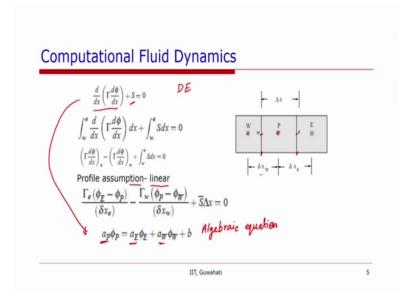
Apart from that so, what is done in finite volume method, what we have here is a simple diffusion equation with source term. So, this is the diffusion term, and this is source term and in finite volume let us say they are 3 adjacent cells for a one-dimensional problem. So, the length of the name of the cells or the cells enters are P which is point W a point on west of it and E a point east of it; the phases are being represented by small W and E small E for west and east sides respectively.
