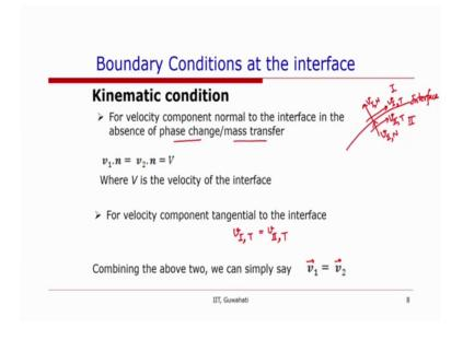
Now, at the interface because when we have 2 phase flow, they have the usual boundaries of the domain plus 1 boundary is the boundary between the 2 phases and this boundary would be moving; it is not a fixed boundary.
