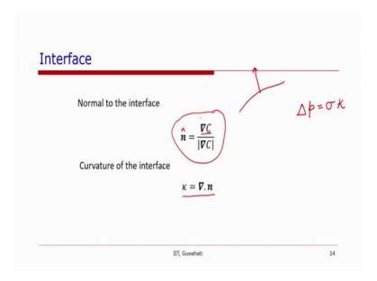
At the interface, when we want to implement something or when we want to implement the surface tension force, then we need the curvature. If you remember the pressure jump at the interface or Laplace spacer is defined as sigma kappa; where kappa is curvature of the interface.
