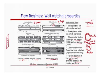
Now another point that is very important in micro channels that the properties of the channel walls. The channel walls it might be hydrophilic hydrophobic. So, hydrophilic means it likes the water and hydrophobic means it does not like the water. So, that means, there is in the hydrophilicity and hydrophobicity that comes into picture only when there is a 3-phase contact line. So, on one side you have liquid another side you have gas so, because and that that will depend on the contact angle.
