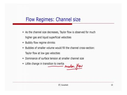
Now, another effect the effect of channel size. So, edge we have seen that the bond number it is value decreases as the channel size decrease. And there will be a significant difference between the bond number at 1 mm and bond number at 10 mm to be precise it will be about 10 to the power minus 4. So, the 4 order of magnitude difference at 2 different, 10-micron size, and 1 mm or 1000-micron size, there will be very large difference in the bond number.
