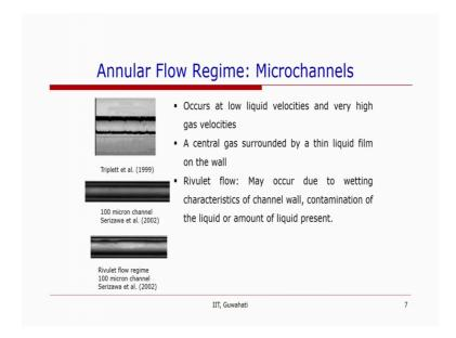
Then finally, we have annular flow regimes of and the gas velocity is increased further. When get the bubbles have merged the waves have subsided, and there is a continuous gas code, and there is a thin liquid film on the wall. So, this occurs at low liquid velocity and very high gas velocities.
