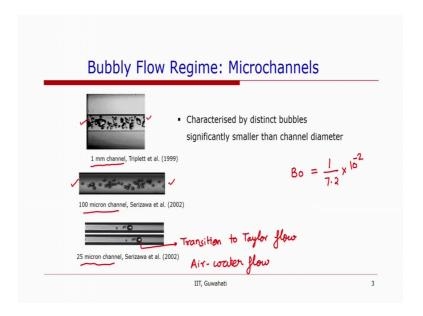
So, let us define the flow regimes one by one. So, the bubbly flow regime, I have put 3 pictures from 3 different publications or 2 are from the same publication actually. So, this is the bubbly flow in 1 mm channel, in 100-micron channel and 25-micron channel all for air water flow.
