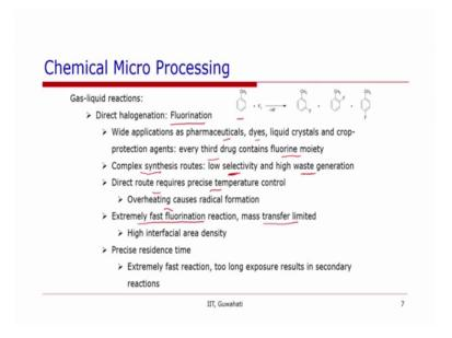
So, one of the most investigated reaction in micro channels has been Halogenations and in particular Fluorination. So, this is for example, Fluorination of toluene because this has wide applications in a number of industries, pharmaceuticals, dyes, liquid crystals crop protection agents.
