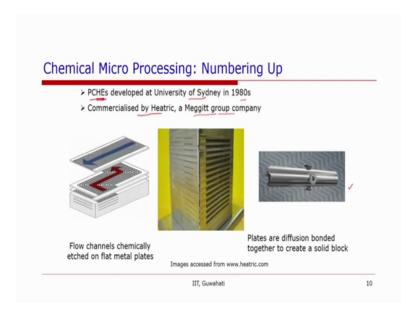
So, one of the issues that often comes up when one is looking at using micro reactors and chemical processing that how to scale up. So, as I have discussed in quite a few times during the course that this is scaling up is achieved by numbering up.
