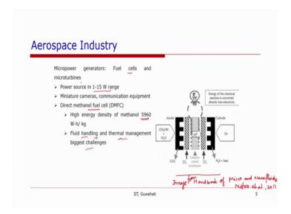
Another application in aerospace industry is in Micro power generators, in the in terms of for example, fuel cells and micro turbines. So, these generators are expected to provide power in the range of 1 to 15 Watt and this power might be required for miniature cameras or mobile applications and other applications where power is required.
