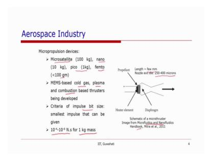
Another application is in Micropropulsion devices. So, with the application of satellite in a number of areas, there have been a thrust towards developing smaller and smaller satellites; so based on that the different names for satellites have also been standardized.
