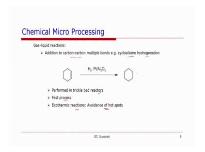
So, by selectivity I mean the yield of the desired product or divided by the yield of the undesired product which is only term generally at selectivity in chemical reaction engineering. Another gas liquid reaction which has been studied it carbon-carbon multiple multiple bond addition for example, cycloalkane hydrogenation.
