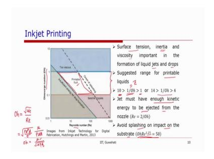
So, now the gas sorge the properties of the material that should be used as printable fluids or that can be used as inkjet. So, this graph is between Ohnesorge number and Reynolds number. We can remember that Ohnesorge number is defined as the root of the wavier number divided by Reynolds number. So, this is equal to the wavier number is rho u square d over sigma Reynolds number rho u d over mu. So, we can cancel out u here and that will be equal to mu over square root of sigma rho d.
