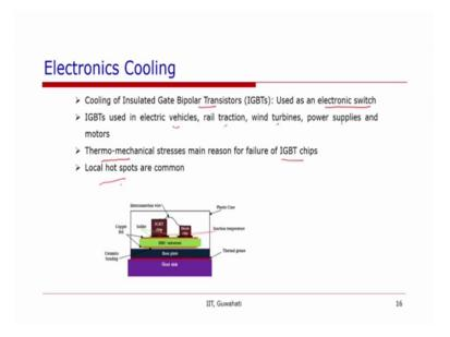
These electronics cooling is also required for example, IGBTs the Insulated Gate Bipolar Transistors which are used as a electronic switches in electric vehicles, rail tractions, wind turbines, power supplies and motors. And it is often observed that the failure of this IGBT chips occurs due to the thermo mechanical stresses which are which might be generated because of local hot spots.
