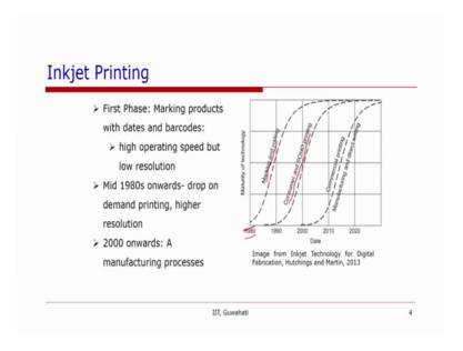
The early developments for the inkjet were about 70s and 80s where, it was developed to mark and code to develop or to have barcodes for the food products or to do the print the dates and prices on the packagings.
