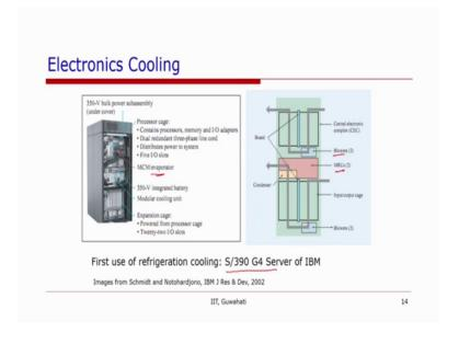
So, here is a image where IBM. They introduced in one of their high end servers or high performance computers and evaporator for the cooling purposes. So, this evaporator this had blowers, but the evaporators were introduced for cooling of some certain components of the system and this was in about 2 decades ago.
