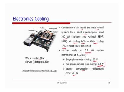
There is another system again by IBM in which the water cooled IBM server has been developed. So, this is based on micro channel and. So, the technology being utilized by INTEL and IBM for the cooling of the electronic systems especially, the computers servers data servers and so on.
