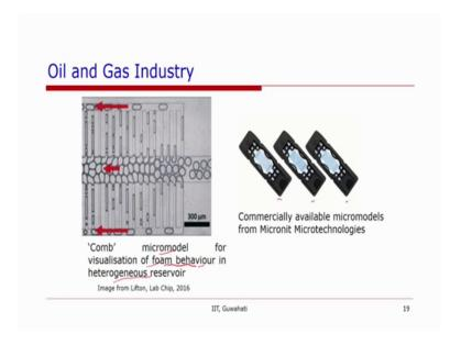
In another Micro model, there is this is say 'Comb' micro model for visualization of foam behavior and heterogeneous reservoirs.
