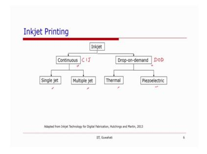
So, if you look at inkjet printing technology, we can divide the technology into 2 or the inkjet printers into 2 different categories. One is Continuous inkjet printer or which is called CIJ in short or Drop-on-Demand inkjet printers or DOD. So, as the name suggests
