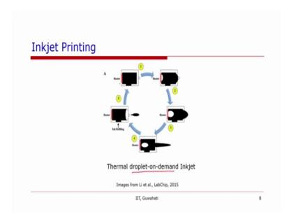
Now, in the droplet on demand the Thermal inkjet printer as the name suggests the technology for the droplet generation is based on thermal magnet. So, the in the jet or in the nozzle, there is a heater and this heater might be placed on a at different positions.
