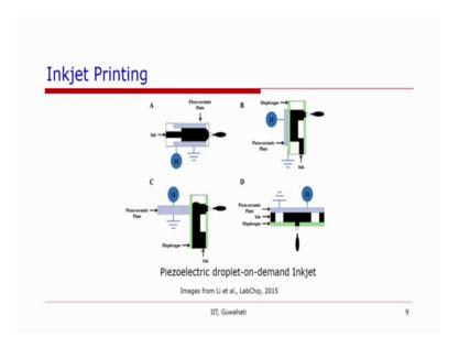
So, this Piezoelectric material is connected with the ink via diaphragm and this podia position can be different as we can see in different images and once, the electric field once we need a droplet, the electric field is applied.
