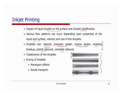
So, once what we have discussed in the technology that drop in the it is continuous inkjet printer, one need to look at the generation of the droplets which is happening by giving perturbation to the jets. And then the travel of this droplet from the print head to the substrate, once it comes to the substrate; then, it is impact on the surface and the droplet solidification are 2 important factors.
