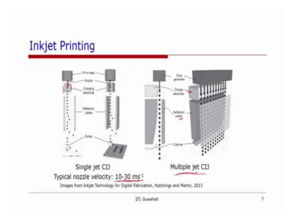
So, in the continuous inkjet printer for the single continuous inkjet printer the jet of the ink and this ink is generally it has a some solvents into it. So, it might behave (Refer
