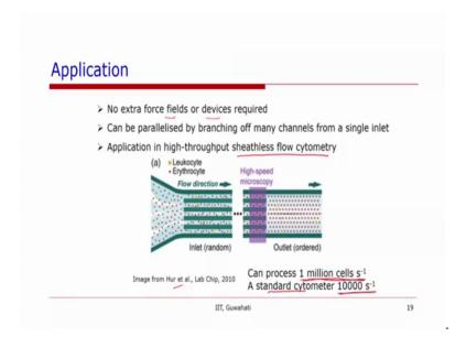
Now, we look at some of the applications of these inertial fluidic effects so, the first application is in C plus flow Cytometry. So, the flow cytometry referred to the focusing of the cells for cells sorting or for cell counting in a number of biological applications.
