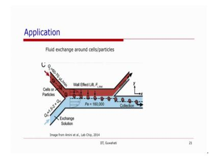
Then the third application is in fluid exchange around cells and particles. So, here the particles are present in one fluid and the particles are exchanged or migrated towards another fluid by so, in this application the rectangular channel was used. So, we have there are 2 focusing positions and by using the different flow rates of the fluid the focusing positions were manipulated.
