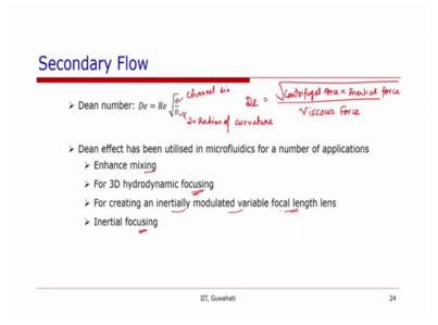
Then there are vertices that are observed at very high Reynolds number the number of vertices are observed to increase. And this effect is characterized by dean number, which is Reynolds number into D by capital D and this D number is ratio of viscous forces and centrifugal force and inertial force small D is channel dia and capital D is 2 into radius of curvature of the curve channel. So, this has been utilized this effect has been utilized in a number of applications in microfluidics.
