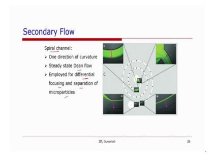
So, there are 2 different kind of curved channels has been used; one in which the channel it is spiral. So, the curvature is in one direction as you can see here and in this case the dean flow will be steady and this is often employed for differential focusing and separation of particles. So, you can see here that the particles separate and moved to a particular position here. So, this is a spiral channels.
