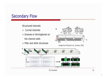
Now, so, till now we have looked at the flow of particles in a structured channel, in a straight channel without any structured in the flow or the channel without any modification in the channel geometry except the cross section of the channel, where the cross section we have looked at the cross section of the channel to be circular or rectangular or square shaped. Some people have also worked with trapezoidal channel and have got some interesting visuals there.
