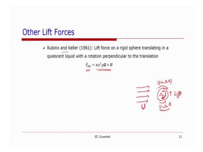
Now, one might also think of some more lift forces for example, a lift force acts on a particle, which is rotating in a uniform flow that there might be a relative velocity between the particle and the fluid.
