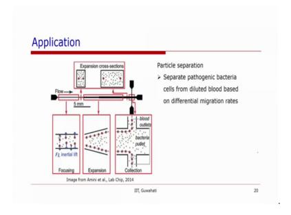
Another application is in the separation of the particles, where the blood cells they are separated from the bacteria. So, the size of the blood cells are larger than the bacteria and due to the inertial force the particles the blood cells, which are significantly larger in size they focused to the equilibrium positions.
