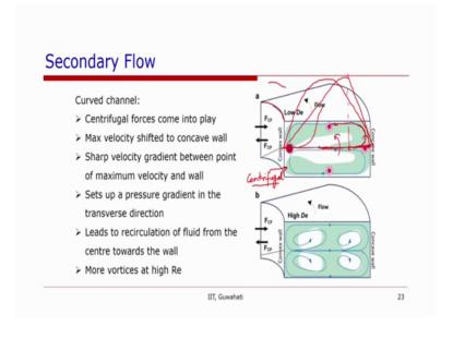
When the flow is the flow happens from say into the page in this direction. So, the inner wall which is the convex wall and the outer wall, which is concave wall there will be a force, which is centrifugal force on the fluid and that force will shift the velocity profile towards the inner wall.
