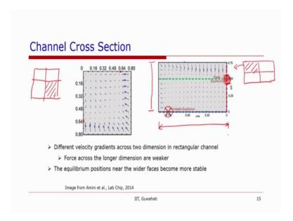
This is explained by Decarlo and others by the magnitude of the forces that act on the particle. So, in a rectangular channel, what it shown here is the force field in a quarter of a channel. The particle experiences similar forces from both the sides of the wall, because the velocity gradient are same. So, the particle focusing position it is somewhere in one of the there will be one focusing position here and another focusing position somewhere here.
