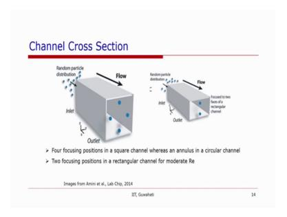
Now, looking at the effect of the cross section of the channel so, in microfluidics it is often convenient to have the channels, which are rectangular in shape or square in shape. So, what we have seen till now that there are focusing positions or there is because the geometry of a cylindrical or circular cylinder is symmetric about the axis. So, the particles will focus on a annular the location and, but in a rectangular channel it is not so, obvious.
