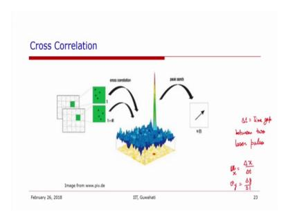
So, using this technique one can obtain the delta x and we already have we already know delta p is the time gap between 2 laser pulses and delta x is estimated from the or cross correlation of the 2 images.
