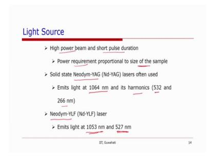
Now, so, the lasers this would have high power beam and sort pulse duration. So, the power requirement that is proportional to the size of the sample larger size more power is required. Now the 2 most often used lasers are Neodym-YAG laser and Neodym-YLF laser these lasers emit lights at the Nd-YAG laser they emit light at 1 0 6 4 nanometers and it is harmonics of 532 nanometer and 266 nanometers generally it is 532 nanometers that is used in the application.
