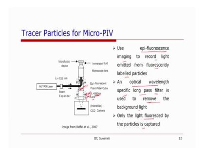
So, generally what is done in such cases or specially for micro PIV that a in place of the direct imaging one uses epi-fluorescence imaging to record light from the fluorescently labeled particle. So, the particles they are labeled flow by fluorescence. So, the particles are fluorescent particles and an optical wavelength specific long pass filter is used to remove the background light.
