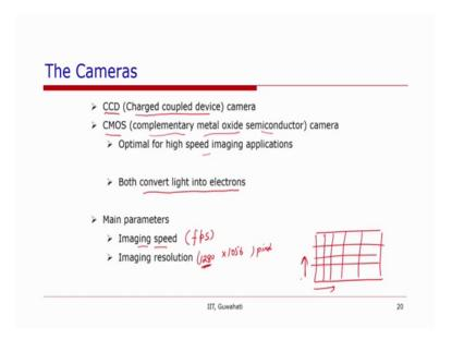
Now, the 2 things that we have discussed at the case of particles and the light source and the optical seat, if required or the volume illumination of the flow, now these images nowadays in most of the PIV applications these images are captured using either a CCD camera or a CMOS camera; both of these cameras convert light into electrical signals. So, CCD camera is charged coupled device, which goes and gives very good and accurate a special resolution.
