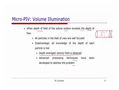
So, now the 2 cases can be there that when the depth of field of the system exceeds the depth of the flow. So, in this case what will happen that all the particles that are there in the field of view they will be illuminated, because all the particles are well focused. So, one will not have an idea for example, in a when one has a light sheet optics then a particular plane is illuminated.
