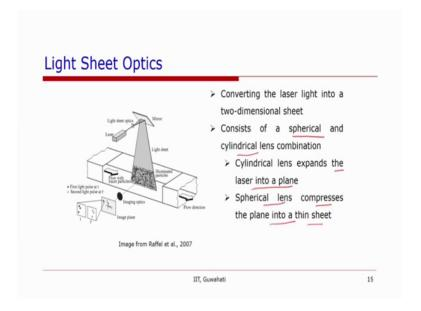
So, this laser is converted into a light sheet optics using a combination of a spherical and a cylindrical lens. The cylindrical lens expands the laser into a plane. So, that converts a laser into a plane and this a spherical lens it compresses the plane into a thin sheet. So, that is required for PIV applications in conventional channels whereas, the illumination is not a sheet illumination in micro PIV or to analyze the flow micro channels it is volume illumination as we have seen before.
