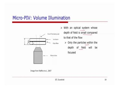
The other option is that one has an optical system whose depth of field is smaller, when compared with depth of the flow. So, only the particles that are there within the depth of field will be focused. So, in a volume illumination rather than the illumination the depth of the field from the optics are the from the objective lens is such that that if particular region in the channel is focused and of that particular region, the images will be obtained or they will be having a high intensity.
