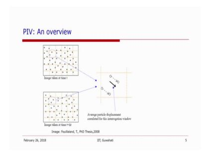
Now, these 2 images which are taken at time T and time T dash which is equal to time T plus delta T they are cross correlated and from that the average displacement of the particle is obtained for each interrogation window. So, the local velocity field in the each interrogation window is obtained by cross correlation technique.
