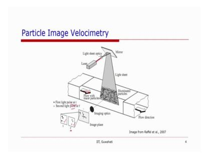
So, this is a typical schematic of a PIV setup, you can see that this is the test section in which the flow is happening from in this direction and this flow is seeded with the tracer particles. Now the laser light is introduced on it and you can see this that the laser light in a 2 d PIV system for a conventional channels or large channels the laser light is converted using light sheet optics it is converted into a light sheet.
