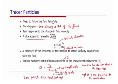
Now, we let us look at these components one by one. So, the tracer particles if they do not have the same density as that of the fluid, then the because of the buoyancy the particle will have a motion of their own in the fluid. So, it is often advisable that the particles are non-buoyant or so, they have the same density of as that of the fluid fast response to change in the fluid velocity.
