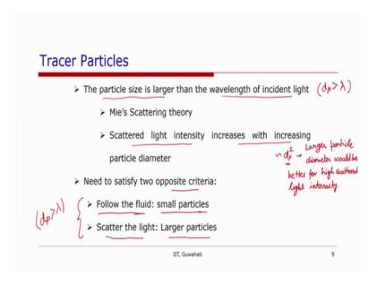
So, looking at the Mie's scattering criteria which is when dp is greater than lambda, when the particle size is more than the wavelength of the incident light, it has been observed that the scattered light intensity increases with increasing particle diameter it is probably proportional to dp raise to the power 2.
