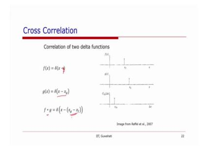
So, let us say for fx is equal to delta x minus xf the first function, which is a delta function. And another delta function gx, which is given as x minus xg the multiplication of 2 is given by a x minus xj minus xs. So, one can get the displacement as xj minus xf. So, one gets a peak here.
