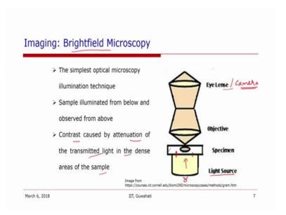
So, the bright field microscopy is that a light source emits the light from the bottom. So, the test section is here and the light is emitted from the bottom and it is visualized either through eyes or a camera. So, of course, when we want to do the measurements and recorded we need a camera.
