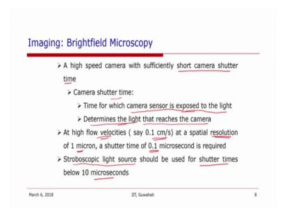
So, for those who do not know what the camera shutter time means, it is the time for which a camera sensor is exposed to the light when the picture is being taken. And this determines the exposure time it will determine the light that will reach the camera.
