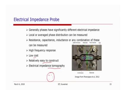
So, the other technique that can be used apart from imaging and refractive index change is based on the change in the electrical properties of the two fluids that when one fluid say gas and liquid they have a very different electrical conductivity or resistivity or electrical capacitance.
