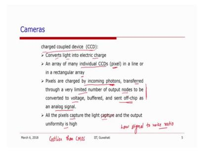
So, CCD camera is based on a charged coupled device which is in short is called CCD. So, the CCD camera converts the light into electric charge, based on the photoelectric effect and the CMOS sensor is also based on the same principle.
