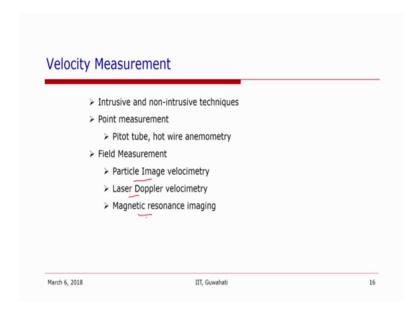
So, some of the popular techniques are particle image velocimetry and the related technique particle tracking velocimetry, then laser Doppler velocimetry, and MRI or Magnetic Resonance Imaging. We will discuss micro PIV or Particle Image Velocimetry in a separate lecture.
