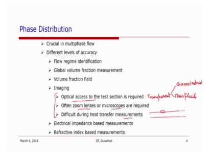
So, for the phase distribution of course if one can image the system then one can get the phase distribution. So, for imaging one needs optical access to the test section, by optical axis I mean the test section should be transparent.
