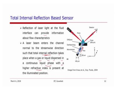
So, one of the techniques that have been developed is that the reflection of laser light, at the fluid interface it can provide the information about the flow characteristics.
