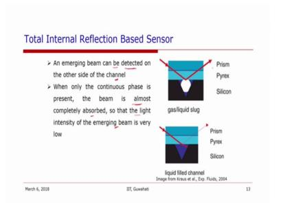
So, by detecting the emergent beam on the other side of the channel; one can obtain the phase distribution. So, when only the continuous phase is present, the beam is almost completely absorbed there is no nothing happens.
