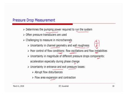
Now, coming to the pressure measurements the pressure measurements is a difficult bit, but it is very important bit because it is required to determine the pumping power to run a system. So, it is always required to design a system efficiently, one need to have an idea about the pressure drop that happens in channel. Often pressure transducers pressure transducers, which can capture the low changes or small changes in pressure are used
