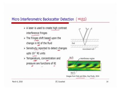
Now, another technique, which is known as MIBD or Micro Interferometric Backscatter Detection so, in this case a laser light is used to create high contrast interference fringes. And the shift in fringes is based upon the change in refractive index of the fluids. So, because the two fluids will have different refractive indices so, based on the fringe shift one can measure the change in the refractive indices and change in the properties of the fluid.
