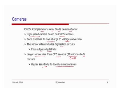
So, they have the semiconductor sensors and again these semiconductor sensors they has they have it is own charge to voltage conversion devices. And so, each pixel or each sensor has charge to voltage conversion device and then this sensor itself has a
