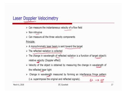
So, it has a brief discussion of laser Doppler velocimetry, in this technique like micro PIV; it is also non-intrusive and it measures the instantaneous velocity of the flow fields.
