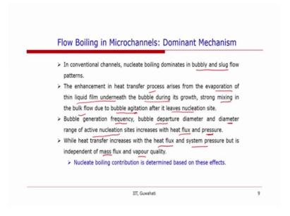
Now, in conventional channels the nucleate boiling it dominates in bubbly and slug flow patterns and the enhancement in heat transfer occur from different physical phenomena such as evaporation of the liquid film that is near the bubble and the bubble growth and then this causes strong mixing in the bulk flow because of the bubble agitation when it leaves the nucleation site. So, that is the enhancements or those are the factors which causes the enhancement of heat flux during nucleate boiling.
