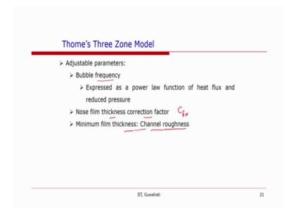
And the minimum film thickness. So, they were able to eliminate one of the fitting parameters channel roughness or based on the channel roughness. So, this is not arbitrary anymore. However, the parameters for the bubble frequency and the film thickness correction factor. So, there are four parameters that needed to be determined from the experimental data.
