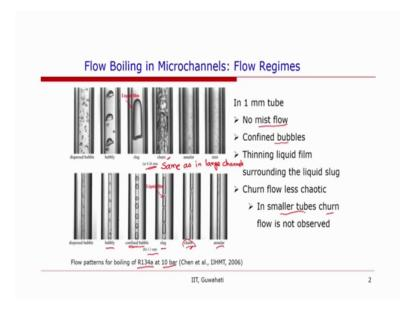
What we have in this slide is; the experiments that have been performed in two different channel sizes: one is 4.26 mm and the other one is 1.1 mm and this is for boiling of R 134 a at 10 bar pressure and they observed that while the boiling regimes in 4.26 in mm channel they looked like conventional channel whereas, there was significant difference in the flow regime maps that were observed in the millimeter or 11 millimeter size channel.
