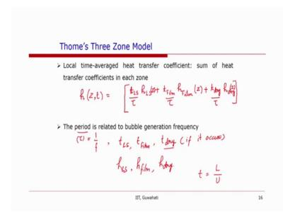
So, they considered the heat transfer for such a case and calculated that the heat transfer or the local heat transfer at is equal to sum on the heat transfer coefficients in each of these three zones. So, 1 over tau t of liquid slug h liquid slug plus t of film h of film z plus t of dry zone into h of dry
