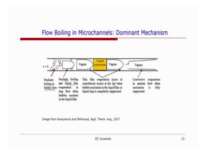
This is a visual picture of such that at low when the vapour quality is low, then bubbly flow occurs and the nucleate boiling is observed at higher vapour quality nucleate boiling as well as liquid film evaporation in slug flow both occurs even bubbles also nucleate in the liquid film. Further, on the evaporation in the thin film occurs and most of this contribution comes at the tip of the bubble and as the quality is increase the annular flow is observed.
