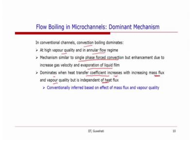
On the other hand, in the convection boiling of which occur at high vapour quality and the flow regime is annular flow regime nucleate boiling is almost suppressed there is less number of bubbles and the mechanism of heat transfer in this case is similar to single phase forced convection and the enhancement occurs, because of evaporation of liquid film and the increased gas velocity.
