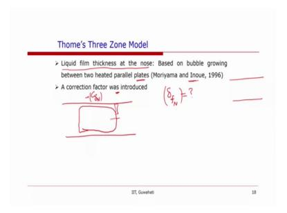
So, now the next question is that we need to find out the film thickness and from that we can obtain a relationship for the rate of evaporation of the film or the decrease of the thickness of the film with time using energy balance. So, first thing is that we need an expression for the liquid film thickness at the no jump the bubble. So, if this is our slug zone then what is the thickness of the liquid film at this point.
