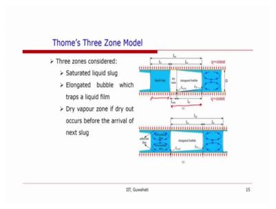
So, this is a visual picture of their model they considered three zone the liquid slug and the bubble which evaporates. Now depending on the length of the bubble and the velocity and wall heat flux there may be 2 or 1 region. So, as we see in the upper image there are two regions that the bubble the film surrounding the bubble has dried out; where as in the image below the film remains always surrounding the bubble. So, one
