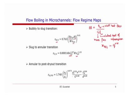
So, the transition from bubble to slug regime it depends on liquid only Reynolds number and this is gas only waiver number boiling number. So, boiling number which we have not seen until now is defined as Q wall G h Lv. So, Q wall is wall heat flux G is mass flux and hLv is latent heat of vaporization.
