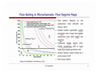
So looking at the 4 flow regimes that they identified IB which is isolated bubble regime, so this is characterized by that the generation bubble generation rate is larger than the coalescence rate of the bubbles and in this case they saw both bubbly and the slug flow.
