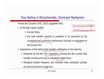
Now, when the vapour quality is high then the flow regime is annular flow regime and or in such case the heat transfer is expected to govern by the convection and conduction in the evaporation of thin film. So, in the annular flow there is a thin film that will reduce in the thickness because of the evaporation of the thin film. So, the conduction through the film and the evaporation will be the; dominant mechanism.
