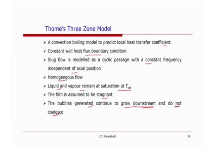
So, now based on he is under physical understanding develop from the experiments and cfd simulations Thome's he proposed a three zone model to explain the boiling in the slug flow regime and he had the following assumptions that the wall the boundary condition on the wall was a constant wall heat flux boundary condition and slug was considered as a cyclic path passage.
