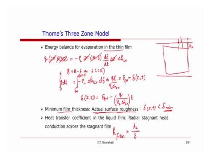
Now, based on the energy balance and expression was obtained for the evaporation in the thin film. So, for the bubble region we have the film thickness here as delta n and when it passes through the thickness of the film keep decreasing. So, if we consider a delta Z length of the film then we can apply a heat balance that q 1 pi r where r is the radius of the channel delta z.
