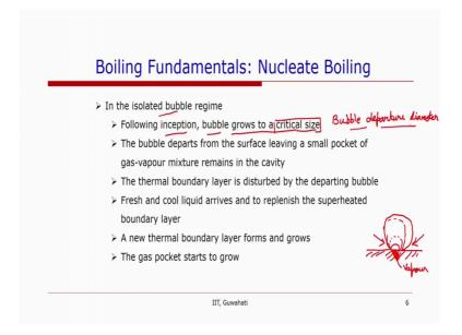
So, when there is one isolated bubble what happens that in the, in during the heterogeneous bubble nucleation after the boiling inception the bubble start growing and then it grows to a critical size; which is generally called the bubble departure diameter. So, this critical size is known as. Then when the bubble has grown to a sufficient size the bubble departs from the surface. So, it leads the solid surface with so if we have a picture of a nucleation site.
