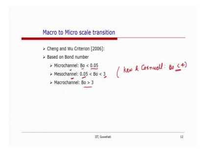
Then another criteria based on the bond number was suggested by Cheng and Wu. So, that was based upon the bond number itself and the bond number if it is less than 0.05 then the termed it has microchannel and between 0.05 to 3 it was termed as mesochannel and bond number greater than 3, this was termed as microchannel. So if we look at the Kew and Cornwell they had bond number less than 4 for the microscale effect to assume importance.
