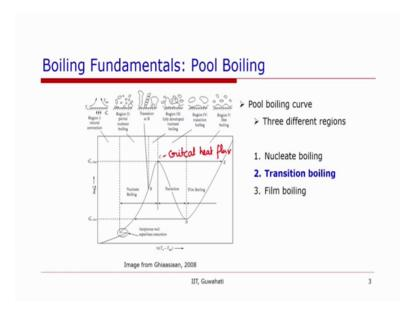
Now, moving on after the nucleate boiling at this maxima point C is called where what we have is critical heat flux. So, at this heat flux the surface is intermittently covered by vapor. So, most of the surface is covered by the vapor phase and the conductivity of vapor is smaller than that of liquid and then so we have very little heat transfer when you compare with the nucleate boiling region.
