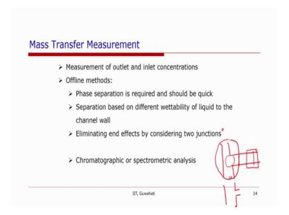
Now, when the experiments are conducted different methods are used to measure the mass transfer. So, mass transfer will be basically measured by measuring the concentrations either locally or at the inlet and outlet. So, every time we want to do the there are two different methods one is offline method. So, for the offline method one take a sample or one has the known concentration at the inlet and then the concentration at the outlet has to be determined.
