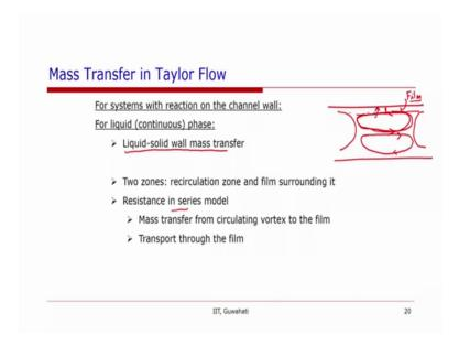
So, one need to look into all these cases now for systems with reaction on the channel wall so what we have looked at is gas to solid mass transfer. Now another important mass transfer that one need to look at from liquid to solid.
