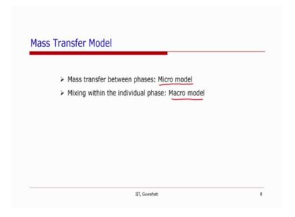
And now we will look at some generic features of the mass transfer models. Now there can be or there are two different kind of models because one need to look at the mixing within the phase itself once the transfer through the interface has happened then the solute or the liquid or the gas phase will mix in the liquid phase so that comes under macro model so, that is mixing within a phase.
