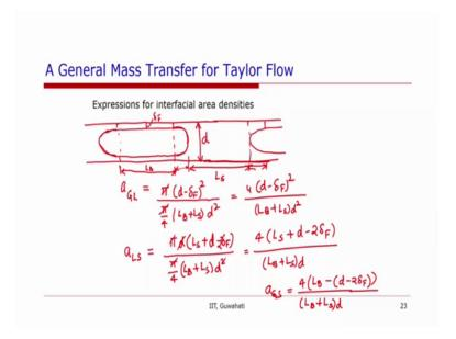
Now, these because the bubbles can be approximated so one can easily get an idea of the geometries or the interfacial area densities in these cases. For example, for the a G L case where G L is the interfacial area density of the caps.
