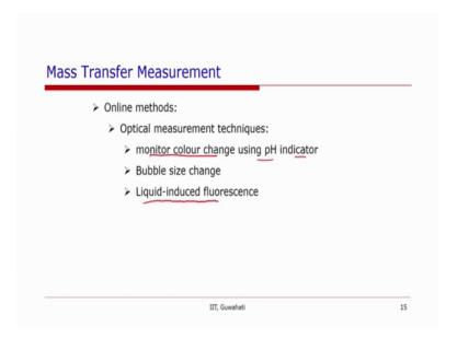
In the online measurement most of these online measurement techniques which means that the concentration is being measured as the fluids move in the channel so, these online measurement techniques most of them are based on the optical measurements.
