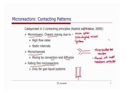
So, coming back to micro reactors specially for gas liquid or liquid liquid flow Kashid and Minisker I think I have a spelling mistake here. So, Kashid and Minisker they divided the micro mixers into or micro channels or micro reactors into three different categories based on the contacted principles micro mixers, micro channels, and falling fault film reactors.
