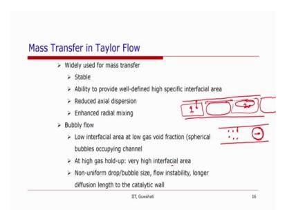
So, now coming to mass transfer in the Taylor flow regime it is extensively used in most of the mass transfer applications in micro channels for gas liquid or liquid liquid flow. Taylor flow regime or the segmented flow is one of the most popular flow regime in
