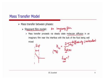
So, looking at the micro models which are the specific to two phase flows there are different models that are being used. So, the first one is stagnant film model so it assumes that there is a, at the interface there is a stagnant film which is imaginary.
