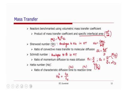
So, some more basics about the mass transfer the reactor because the mass transfer is a function of mass transfer coefficient as well as the interfacial area so, the reactor performance is generally given as k multiplied by interfacial area density. So, it may be a so a k gas to liquid interfacial area gas to liquid. So, a specific interfacial area that is interfacial area per unit volume meter square per meter cube k has unit of meter per second.
