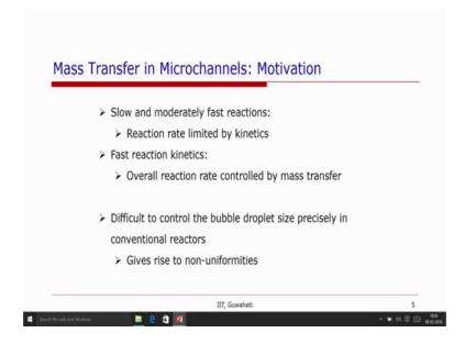
So, contacted between the phases is important because the mass transfer between the two phases happens by the interface so it is important to have a large interfacial area ok. So, that is where we have a micro channels coming to picture.
