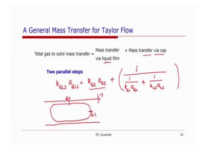
So, one can write that the total gas to solid mass transfer or k let us say G L S into a G L S will be equal to there are two parallel steps that the mass transfer happens via the liquid film and mass transfer via cap.
