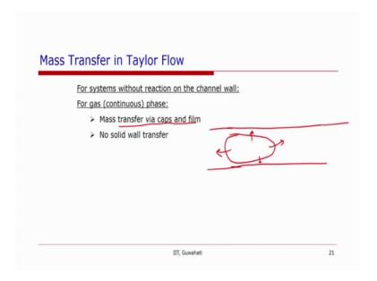
So, what we have looked at is mass transfer in case where there is a gas solid liquid system and reaction is happening when there is no reaction on the channel wall then one just need to look at the mass transfer.
