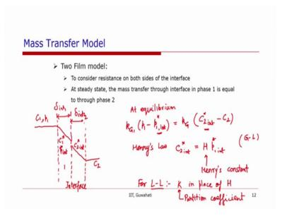
Now, consider the mass transfer at an interface. So, if this is the interface between two phases and if we consider that there is considerable resistance on both sides of the interface so we plot the films surrounding this and this is delta int 1 we can call in phase 1 and this is delta int 2.
