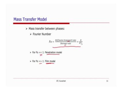
It has been suggested that the choice of the penetration model and film model can be determined by a non dimensional number or Fourier number which is defined as the ratio of diffusive or molecular diffusion divided by the storage depth.
