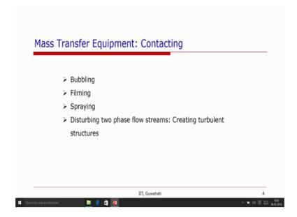
So, the contacting pattern in these reactors may be by bubbling as we have seen in bubble column or a film reactor filming or a spring. So, by a spraying the small droplets of the mass transfer can happen of say for example, further when the drying of milk formation from milk to milk powder this kind of electrodes are used and say another application can be the coating of different pharmaceutical granules etcetera.
