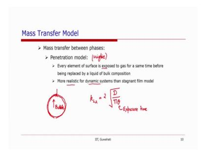
Another approach that is used is called penetration model and this is due to Migbie and so in this basically what it suggested that each liquid elements take the same time in contact with the fluid or each element of surface.
