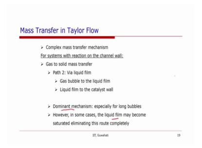
This is thought to be a dominant mechanism especially when the bubble is longer than the interfacial area of the film region will be large compared with the interfacial area and those caps.
