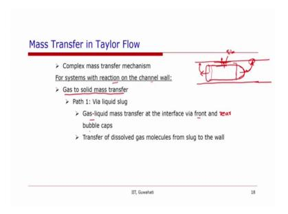
So, the mass transfer mechanism in such cases will be a can be complicated. So, let us look at the mass transfer we have the systems have reaction on the channel wall. So, if
