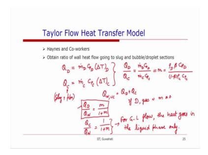
So, based on this we can write the heat flux Q by the dispersed phase is equal to m dot dispersed phase CPD into delta T of dispersed phase. Similarly the Q for slug will be equal to m dot slug CP slug or we can say, because what we are looking at rather than slug we are looking at, here is the continuous phase which is slug plus the film. So, m dot c is CPC delta T continuous phase
