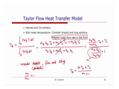
Now, we define the bulk temperature. So, bulk mean temperature can be defined as integral per unit cell rho u Cp Tdv divided by integral for a unit cell rho u Cp dv. So, in an average, we can write this, because rho u is rho udv refers to the mass flow rate. So, we can write in the sense m dot for the dispersed phase. Actually we can consider three phases or consider three zones, consider droplet or bubble film and slug
