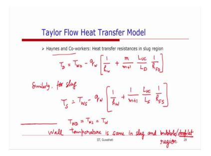
So, when we substitute this, then we will have temperature of droplet is equal to T wall d minus qw 1 over hw plus m over m plus 1 Luc over ld 1 over h F droplet. Similarly for slug one can write T slug is equal to T wall slug minus q w 1 over hw plus 1 over m plus 1. So, we have this as because now it is slug. So, the heat will be 1 over m plus 1 and you see over Ls 1 over h as slug ok. So, we have a relationship between the temperature differences and all this.
