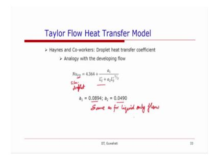
Using similar arguments they have also obtained a relationship for the, this is not fully developed. So, this is film to droplet. So, the Nusselts number is 4.36 for the same correlation, but a 1 and a 2 these are same as for liquid and the flow ok. So, one can obtain Nusselts number for the liquid only from this correlation, and then it is become system of equation becomes closed. So, one can calculate the overall or over all Nusselts number for a in a unit cell in the Taylor flow regime
