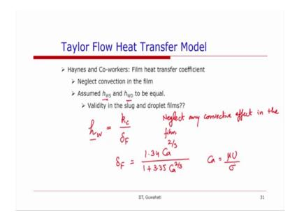
So, as we have already discussed that we have assumed in this case, that the wall heat transfer coefficient for the slug and the droplet regime is assumed to be same, and we can consider only conduction. So, hw is equal to k over delta film, where k is the thermal conductivity of the convective phase. So, we neglect any convective effect in the film. So, the pure conduction will give heat transfer coefficient is thermal conductivity divided by the diffusion length.
