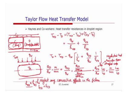
So, now we will be looking at the heat transfer in the droplet regime. So, the picture that we have in this case, is like this. We have a continuous film in which there is a stream of continuous phase, which is slug and dispersed phase which is drop or bubble move. Now we can treat this, the films in the slug and drop.
