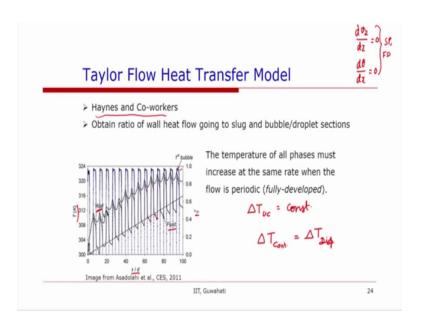
So, that correlation which can be used or a system of equations which can be used to predict the overall heat transfer in a unit cell for fully developed asset number in a channel.
