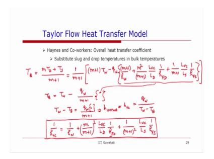
Now, next that the substitute this slug and droplet temperature in the bulk temperature. So, we had this bulk temperature Tb is equal to m TD plus Ts divided by m 1 plus 1. So, we can substitute the two values from here, and we will get m over m plus 1. So, we can write this is 1 over m plus 1 and we will have m plus 1 Tw
