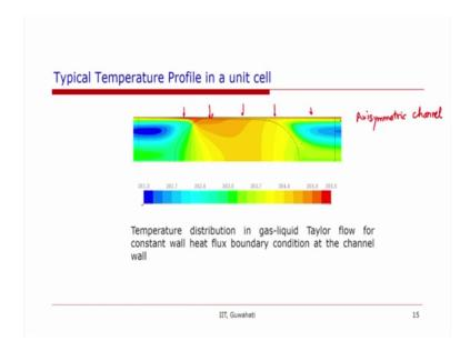
So, let us look at some of the results, this is a typical temperature profile in a unit cell. So, why you see her from the bubble, because an axisymmetric channel, then this is from a d f d computational, where this is done in an axisymmetric channel the. The black line shows the boundary of the bubble, the other bubble will be on the bottom half and you can see the temperature, there is a constant wall heat flux boundary condition
