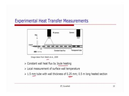
So, the another test section that has been used by walls at all, it is a similar test section and they have made sure. Here actually they have also made sure that the flow is hydrodynamically fully developed, and then there is heat being applied on it, and this heat is being applied by joule heating, and the local measurement of surface wall temperature is being done and using an IR camera probably..
