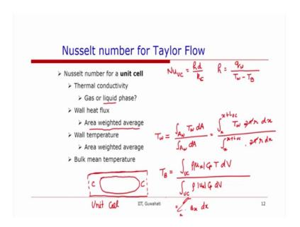
Now,. So, for design calculations we also need to have overall Nusselt number, now because Taylor flow is periodic. So, if we consider the flow, when the heat transfer also have become periodic, then we can analyze flow in one unit cell which consists of one bubble or droplet and the slug around it. And once we have obtained this we can use the same Nusselt number for the entire channel..
