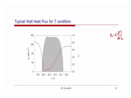
Now, this is a typical wall heat flux for T for the constant wall temperature boundary condition. So, you can see that the wall heat flux is high in the liquid slug zone, and it is small in this region, because that that will be q 1 is equal to k d T over d r at the wall. So, the temperature difference will be small in this region now. So, the heat flux will be small ok.
