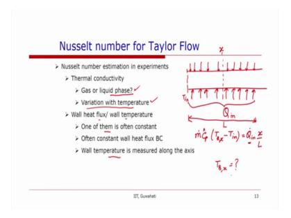
Now, so in the experiment the Nusselt number estimation is done, based the axial lengths. So, if this is the channel from where it is being heated, the channel wall is being heated and the total heat flux to this is, let us say Q in. So, we can write a heat balance at a location x from inlet. So, it can be written as m dot c p and m.dot C p is for 2 phase and T B x or bulk temperature at x location minus T inlet, where T inlet is the temperature at this location is equal to Q n x y L.
