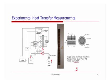
So, this is a typical experimental setup in which the liquid is coming from a liquid tank, and the gas nitrogen, gas is being supplied and then the inlet flow temperature is being measured. Then they come into a mixing section and the fluid move along the test section, and the temp, wall temperature is being measured at different sections. The wall is being heated A by A power supply..
