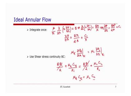
Now, the equation, if we look at this equation again, mu over m r del over del r are mu over r, del over del r, del v over del r is equal to minus del p by del z or d p by d z, which we have named as B now. So, we will have, when we integrate this equation, we will get del r, r del v r over del r is equal to B R over mu which will give us Del, sorry, this is not v r, del v over del r is equal to this, will be r and this will be equal to B R square over 4 mu.
