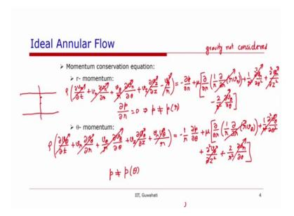
Now, let us come to the r momentum equation. So, for the cylindrical coordinate, the r momentum equation is rho del v r over del t plus v r, del v r over del r plus v theta over r, del v r over del theta plus v z, del v z over del z minus v theta squared over r is equal to minus del P over del r plus mu, del over del r 1 over r, del over del r of r v r plus 1 over r squared del 2 v r over del theta 2 plus del 2 v r over del z 2 minus 2 over r squared del v theta over del theta.
