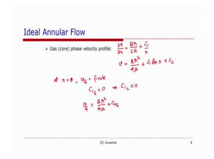
So, we will have del v over del r is equal to B r over 4 mu plus C 1 by r, when we integrate, we get v is equal to, sorry, this is, this will be B r by 2 Mu. So, when we integrate this further, we will have B r squared over 4 mu plus C 1 l n r plus C 2 and now, we can write the same equation for gas phase and liquid phase.
