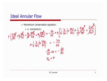
When we write the z momentum equation Rho del v z over del t plus v r, del v z over del r plus v theta over r, del v z over del theta plus v z del v z over del z is equal to minus del
