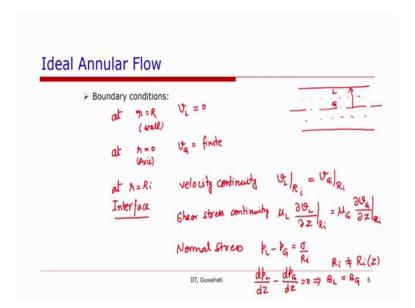
So, we can write this equation later on for both the phases. Let us look at the boundary condition. So, the configuration we look at again. So, this is our interface in the centre. So, at r is equal to capital R, which is general wall. We will have v of liquid, because this
