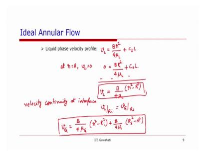
For liquid phase again, we can write the same velocity profile. So, if C 1 G is equal to 0, this will make C 1 L is equal to 0 too. So, we will have v L is equal to B r square over 4 mu L plus C 2 L and at r is equal to capital R, that is at the wall, we have a v L is equal to 0. So, the substitute 0 is equal to B capital R square by 4 mu L plus C 2 L.
