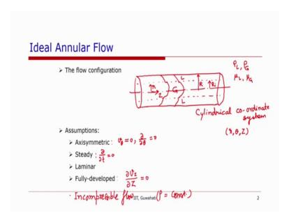
So, let us draw a configuration of an ideal annular flow. We have a channel. Let us say this is a cylindrical channel and in this cylindrical channel, the interface is located somewhere here. So, this is phase 1. Let us consider gas liquid annular flow.
