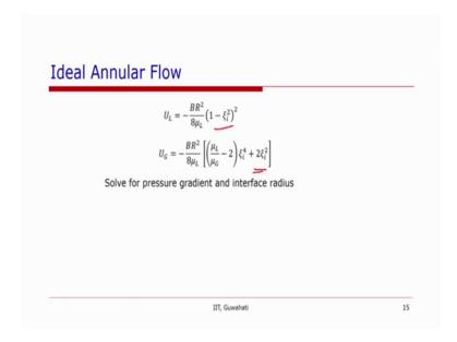
So, we can look at this in the ideal annular flow, these are the U L and U G, the two phase flow rates and the superficial velocities, which we have solved, just solved for and now, when we solve for pressure gradient and interfacial radius.
