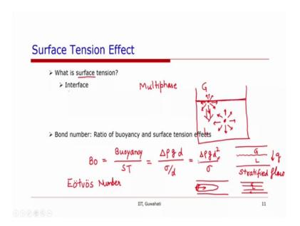
So, what is surface tension? Surface tension of course, occurs at an interface. So, an interface is a boundary between 2 fluids. So, for surface tension to occur of surface tension requires that there is an interface. So, it is an multiphase phenomenon. If there is an interface, then it will have multiphase associated with it.
