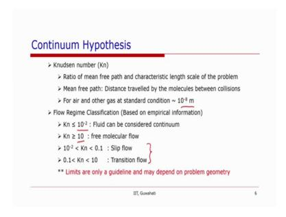
So, if we look at the continuum hypothesis. It is often described or determined by a non-dimensional number, or it can be described by a non-dimensional number which is known as Knudsen number. And this Knudsen number is the ratio of 2 length scale, one is the length scale for the molecular motion which is mean free path of the molecules, and another one is the character length scale of the problem or of the system or of the channel that we are looking at.
