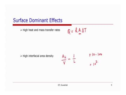
So, and at the same for the same region, you might here that in microchannels, the heat and mass transfer rates are very high. So, if you write the heat transfer rate for convective heat transfer, you will write Q is equal to h A delta T; where A is the area of the surface. So, this area of the surface or the Q is proportional to the area of the surface. Similarly, in the mass transfer the rate of mass transfer is proportional to the area of the surface.
