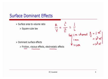
So, In microchannels surface area to volume ratio. So, let us write this surface area as A and volume as V surface area is proportional to length squared. And volume which proportional to L cube. So, we will have this as 1 over L. The ratio of surface area to volume varies with respect inversely proportional to the length. So, for one-meter
