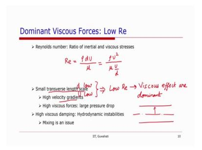
So, viscous force they can be represented by a Reynolds number; which is the ratio of inertial forces and viscous forces or in terms of this the stresses.
