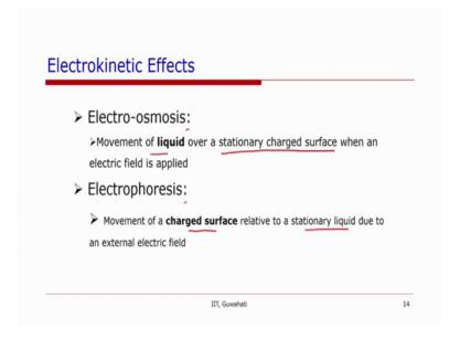
So, electro osmosis is that the stationary charged surface, which is not necessarily it is because of the electric double layer. In general, if the surface is charged and when a electric field is applied, the movement of liquid so, when an electric field is applied on a stationary charged surface and the liquid move, then it is known as electro osmosis. On the other hand, electrophoresis is that a charged surface itself moves related to a stationary fluid, because of an externally applied field.
