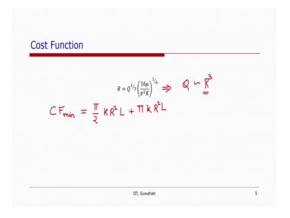
So, this will give us the relationship, which is R is equal to Q to the power 1 by 3 16 mu by pi square K whole to the power 1 by 6. So, that gives a relationship that, Q is proportional to R cube. So, this is the cost function. Now, if we want to find out what is the value of this cost minimum cost function that will be we can substitute the value of Q here. So, if we go back and look at that Q square what is the value of Q square that is 2 pi square K R to the power 6.
