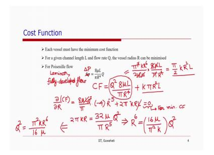
So now, we would like to minimise this energy, because the circulatory system is made up of different these different vessels. So, the total cost will be the sum of the cost function for each vessel. So, it is the minimising of the cost function, is basically it comes down to minimising the cost function for each vessel.
