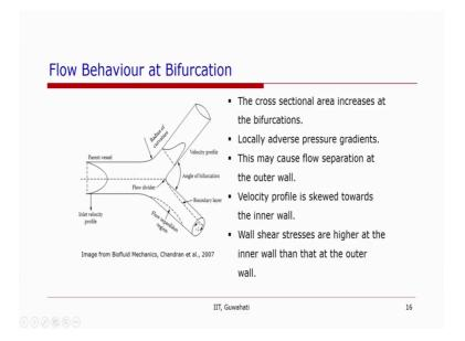
Now, as we have seen just few slides before, that when the bifurcation happens the flow area is going to increase. So, when the cross-sectional area will increase; that means, there will be less or the flow velocity will decrease or there will be locally adverse pressure gradients.
