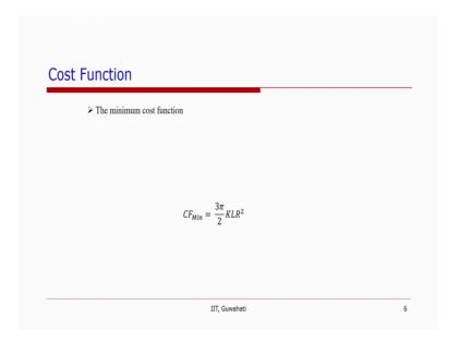
So, the minimum C F will be the minimum cost function will be, 3 pi by 2 K L R square out of which, the operating cost is pi by 2 K L R square and the remaining is the maintenance and generation cost ok.
