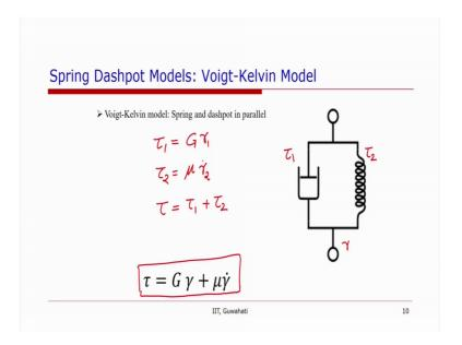
Another combination which is frequently discussed or which is simple model which parallel combination of spring and dashpot. And in such case the deformation will be same in both the cases, whereas they will experience different stresses let us say tau 1 and tau 2. So, we can write tau 1 is equal to G gamma 1, and tau 2 is equal to mu gamma
