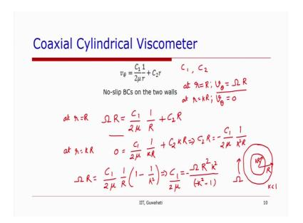
So, if we look at this equation C 1 by 2 mu 1 over r plus C 2 r. Now, we have two constants C 1 and C 2. So, to find out this we need two boundary conditions and these two boundary conditions within will be the no slip boundary conditions on the two walls
