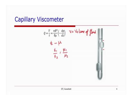
So, one can see that Q which can be written as V over t, where V is equal to volume of fluid generally in a viscometer the volume is fixed between these two points. So, the volume is fixed. Q is equal to V over t pi R to the power 4 by 8 mu minus d p by d z. And so one can see that t is directionally proportional to mu. And if the measurements have been done for a fluid already, then one can just simply use formula t 1 by t 2 is equal to mu 1 by mu 2 to calculate the viscosity of a fluid.
