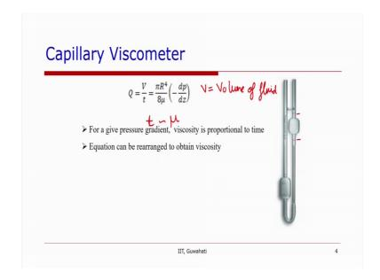
So, this equation can be rearranged to obtain the viscosity.
