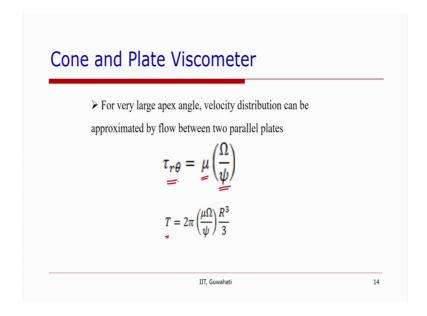
For very large apex angle, one can find out the velocity distribution that and from that the torque and one get that torque is proportional to gamma, and the viscosity is the proportionality constant. So, one can measure the velocity here. And from that one can again calculate the torque. So, this is shear stress and the torque.
