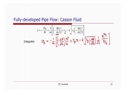
So, let us now integrate this equation, because the right hand side have only r or constants, because yield stress and the pressure gradient both are constant in independent of the radius. So, we can integrate this, to obtain v z is equal to minus 1 over m within bracket minus d p by d z r square by 4 plus tau y r minus 2 root of tau y minus d p by d z. Now, one over root 2 r to the power 3 by 2 divided by 3 by 2. So, if we write this down this is what we get and then integration constant.
