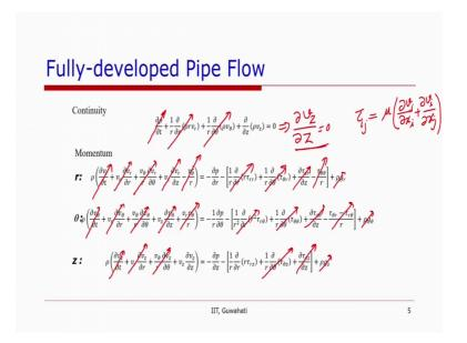
So, let us look at the conservation equation again in the expanded form in cylindrical coordinate. So, what we see here is the continuity and three components of momentum equation r theta and z coordinates and let us try to see different terms in these equations, because flow is a the steady state. So, all the transient term will go to 0 v r and v theta r 0. So, all the term having v r and v theta will go to 0 we neglect body forces now the shear stress is a function of velocity gradient.
