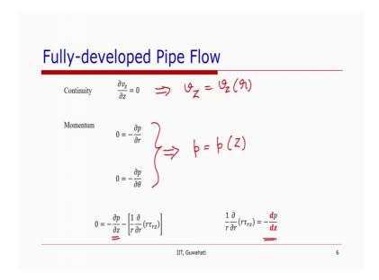
So, if we write down the non 0 terms in all the equations, we will end up this, with this we have already said that if the flow is fully developed then del v z over del z is equal to 0, so; that means, v z is not a function of z. So, from our two assumptions that says that v z is a function of r only, because it was not a function of theta and it is not a function of z.
