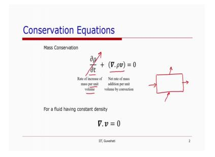
The mass conservation equation is written in this form. The first term in this equation is rate of increase of mass per unit volume, the first term and the second term is the mass that is being convicted or need net rate of mass addition per unit volume by convection. So, if you consider a control volume which might be a part of the channel or a channel. So, the first part represents, you must see here that these equations are in terms of per unit volume.
