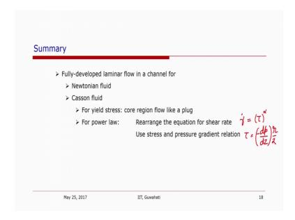
So, in this lecture what we have looked at is flow fully developed flow in a channel for the laminar flow of a Newtonian fluid and of a Casson fluid. In the Casson fluid, there are two things that we should remember that, if the there is an yield stress, then we need to think about that the fluid in the channel will have two region in one region, where the shear rate will be varying across the cross section whereas, in the centre the fluid will flow as a core.
