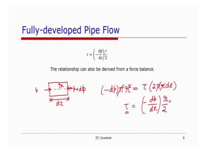
So, this relationship we can also look at a force balance in a channel. So, let us see if you have a fluid element, which has a length of d z and the pressure at the two ends is p and p
