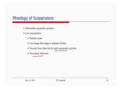
If the particles are deformable and asymmetric and the particles will rotate, they can change their shape, so that the friction is minimised. And viscosity for such case will be lower than for rigid asymmetric particles and because the particles can respond to the fluid. And if the shear rate is or if the shearing is removed then they can regain their shapes. So, they will also show viscoelastic behaviour ok.
