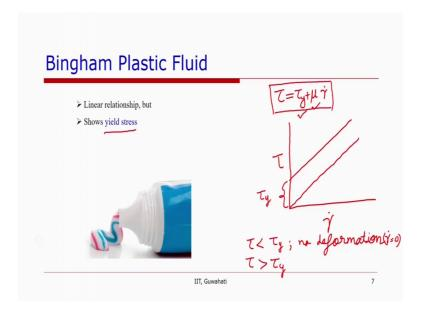
Ah One example is for first fluid that we will be looking at Bingham plastic fluid. So, Bingham plastic fluid, they still have the linear relationship between a stress and rate of a strain. So, we can say that tau is equal to tau y plus mu gamma dot. So, if we plot this on a stress versus rate of a strain plot, then we will get some this kind of behaviour this intercept is known as tau y or yield stress.
