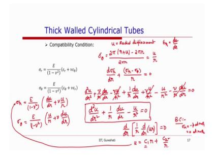
So, if we assume that u is the, radial displacement of the in the tube, instantaneously the local displacement in the tube. So, epsilon r is equal to d u by d r, and epsilon theta will be or the angular strain will be equal to 2 pi r plus u, minus 2 pi r divided by 2 pi r. So,
