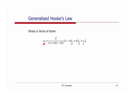
Now, one can also re cast these equations. So, that one can write the stresses in terms of the 3 strains epsilon x, epsilon y, and epsilon z. So, that is (Refer Time: 22:22) algebra and one need to reconstitute or a reframe these equations so, as to obtain shear stress or not the shear stress, but the extra stress normal stress in terms of the 3 strains. So, that is left for you as an exercise.
