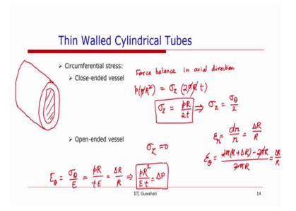
For the circumferential stress if the vessel is close ended. So, for the close ended vessel if we can draw a small schematic of the close ended vessel, then we can do a force equilibrium or force balance, in axial direction then we will have p into pi R square. So, what will be the area the in inner area of the tube that will be a putting a pressure that
