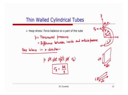
Now, hoop stress we can find by a force balance on a part of the tubes, if we consider a let us consider a semi-circular tube, the thickness of the tube which say t, and the radius is R and we consider a depth of the tube or length of the tube say d z, the internal pressure or p is what we call transmural pressure, which is the difference between inside
