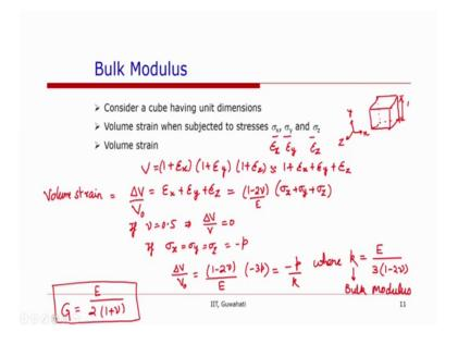
Now, we will look at Bulk modulus. So, Bulk modulus. So, when we consider let us say a cubic volume, and this volume has unit dimension the dimension is in direction is 1. So, the V is 1, now after the stresses in the 3 directions, epsilon x, epsilon y, and epsilon z, the strains are sorry the stresses are sigma x, sigma y, and sigma z. So, the resultant strains are epsilon x, epsilon y, and epsilon z.
