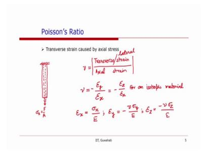
Now, poissons ratio. So, when a rod that first example that we considered when a rod it subjected to a stress a normal stress, then the rod not only it elongates, but to conservate volume the area of the rod also changes. So, there is because of the normal stress, let us say sigma x F over is equal to F over A, there is not only the strain in the axial direction, but there is strain in the transverse direction also.
