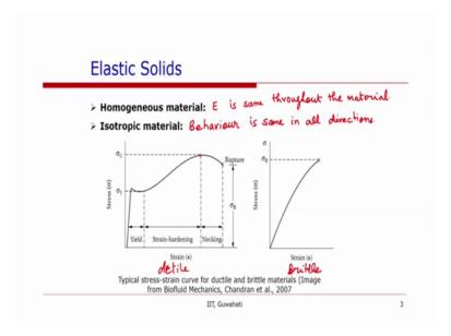
So, homogeneous material means that E is same throughout the bar, or throughout the material that we are considering isotropic material mean that the behaviour or the elastic behaviour is same in all directions, that is if the stress strain relationship is same if we apply is stress in the x direction or we apply a stress in the y direction or the (Refer Time: 06:24) z direction.
