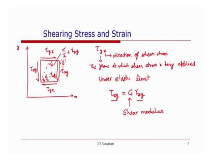
Now, we will talk about shearing stress and shearing strain so, if we consider a planar surface in the x, y coordinate system, let us consider a planar surface. So, in this it is subjected to a shear stress, which is tangential stress tau y x, tau x y, tau x y. So, as we have discussed already in the fluid mechanics review that tau y x has to subscript. So, y is the direction of the shear stress, whereas y is the plane at which shear stress is being applied..
