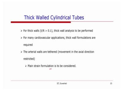
Now, the assumption of thin walled tube is good enough, when the ratio of the thickness and the channel radius is less than 0.1 or so; however, for the thicker a walls, the thick wall analysis needs to be performed and one need to take into account the stress variation in the walls of the tube, for many cardiovascular application this might be the case. So, we will briefly look at the formulation that can be developed for the thick wall tubes, and
