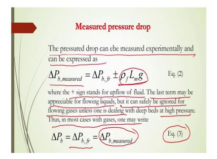
Now, the frictional pressure drop can be measured experimentally which can be expressed as here. This measured pressure drop will be is equal to there are 2 parts of the measured pressure drop you can measure it by a manometer or by any electrical electronics device like you know that pressure transducer you can use that to calculate the accurate pressure drop across the column.
