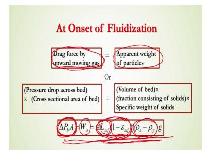
And from this apparent weight of the particles of course, you will get the minimum fluidization.
