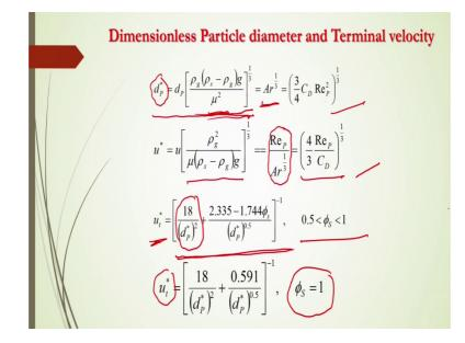
And then we will represent this terminal velocity and also particle diameter as a dimensionless form. What will be the dimensionless particle diameter and terminal velocity why we should do this sometimes some references you will see that it is easier to actually represent the flow resign and also the flow behavior by this dimensionless number.
