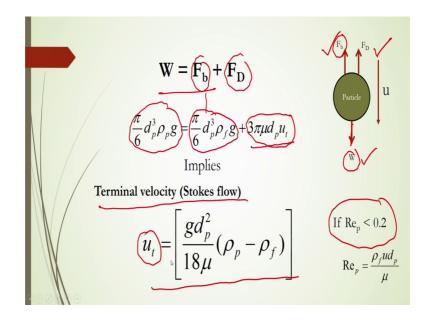
W here if we substitute here for W that will be is equal to pi by 6 d p cube rho p into g and F b this F b. F b will be is equal to this here pi by 6 d p cube rho f into g and then F D this F D is the drag force if we consider it as a under that is stokes flow stokes flow then ah; that means, here if Re p is less than 0.2 then it will be 3 pi mu d p into ut.
