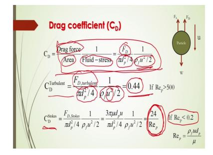
Now, more precisely you can say this drag force will be defined as this drag force divided by area; that means, here projectional area by fluid stress by fluid stress; that means, here this drag force is represented by F D and here projectional is the pi d p square by 4 this is d p is the particle diameter and fluid stress will be represented as by rho f u square by 2. This will be is equal to fluid stress or you can say kinetic energy acting on the particle here.
