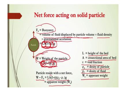
And then what should be the net force acting on solid particle at this minimum fluidization condition you will see here on particle this will be to be fluidized now what are the force now 1 is buoyancy forces acting on this particle and that will be calculated that is volume of fluid displaced by displaced by the particle volume into fluid density and then into gravitational isolation you can calculate the buoyancy force
