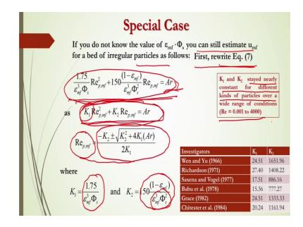
And then if you do not know the value of epsilon mf or sphericity you can still estimate the minimum velocity for a bed of irregular particles as follows in this case you have to first write the rewrite the equation 7 as this here this equation 7 and in this case as I considering or denoting by here k 1 and k 2 this k 1 is defined as here 1.75 by epsilon mf cube into phi s and k 2 will be 1 fifty into 1 minus epsilon mf divided by this epsilon mf q into phi s cube phi s square.
