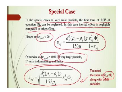
Now, special cases in the special cases of means whether it is very small particles or not of course, you will see in the special cases of very small particle the first term of the right hand side of equation 7 equation 7; that means, see our equation 7 uses see here this equation 7 what is the quadratic equation of the Reynolds number to get the minimum fluidization you will see that the first term of this right hand side of this equation 7 can be neglected for the very small particles.
