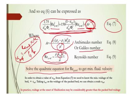
And like this you can simplify this as this equation by 1.75 divided by epsilon M cube into phi s into Reynolds numbers squared plus 150 into 1 minus epsilon F mf that
