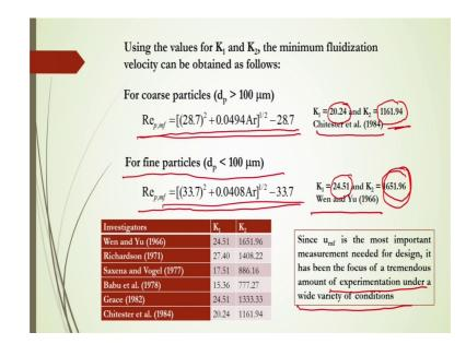
Then you can calculate the minimum fluidization velocity from this equation here in this case k 1 and k 2 are taken from this Chitester et al 94 they got this and it will be k 1 will be equal to 20.24 and k 2 will be equals to 1161.94.
