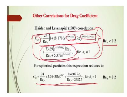
And here see Haider and Levenspiel 99 they have proposed a correlation for drag coefficient and they have represented the correlation as the C D will be equals to 24 by Re p into 1 plus 8.1716 e to the power minus 4.065 into phi s and into Re p to the power 0.0964 plus 0.565 phi s. Here this portion not only this is big correlation of course, some other part here this is 73.69 into e to the power these and divided by Re p plus these.
