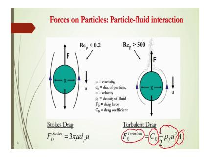
Now, let us discuss about the particle fluid interaction now you will see whenever a particle is flowing in a fluidize bed or it is falling in a fluid medium freely then you will see the liquid and particle there will be interaction now there will be some force acting on the particle whenever it will be moving or falling freely.
