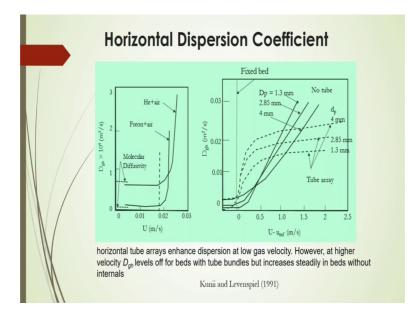
And some results that is given by Kunii and Levenspiel that for that the horizontal dispersion coefficient and for that horizontal dispersion coefficient they have used some horizontal tube arrays for enhancing this dispersion coefficient and they measure quantity of the dispersion coefficient. And they have seen that with increasing gas velocity, initially up to 0.0 or 2 meter per second, the horizontal dispersion coefficient will not change significantly.
