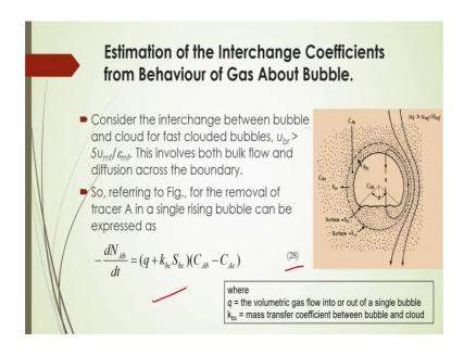
And for this FCC catalyst, Kunii and Levenspiel, they have given this data for how this overall mass transport coefficient will be changing with respect to tube diameter. And estimation of the interception from the behavior of the gas about the bubble also you can calculate from this equation 28 here given in this equation.
