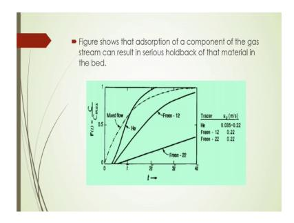
This figure shows that the adsorption of a component a of the gas stream that can results in the series of holdback of that material in the bed.
