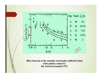
In this case you will see also that mass transfer coefficient will change with respect to a tube diameter.
