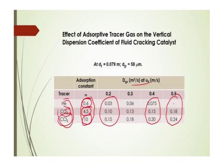
Now, effect of adsorb tracer gas on the vertical position and denoted by the dispersion coefficient of fluid catalytic cracking. So, in that case some observation is given by Kunii and Levenspiel there, if you are using that different tracer concentration then m value will be like this. So, for helium this m value is generally 0.6 for carbon dioxide tracer gas it will be 4.5 and carbon a dichloride it will be is equal to 10.
