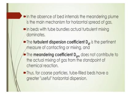
And in the absence of bed internals of course the meandering plumb is the main mechanism for horizontal spread of gas. Now, you can reduce that horizontal spread of gas if you are inserting some tube vertically or you can use the baffle or you can use some other provision. So, that you can decrease a the horizontal dispersion coefficient.
