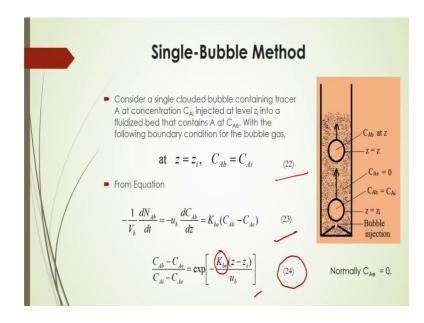
Now, as for single bubble method a, if you are considering that a single clouded bubble and that will contain the tracer A at concentration C Ai which is injected at the level Z, here I into a fluidized bed that contains a at concentration C Ae. Then with the following boundary conditions a given by equation 22, you can obtain this equation 23 and after solution of this 22 this boundary condition you can represent this by this 24.
