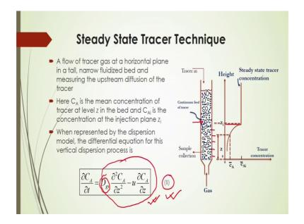
Now, let us see here one important steady state tracer technique here, in this case see the figure described here one a fluidized bed from the bottom gaseous moving upward, and from the top one tracer gaseous allowed to in and allow to mix inside the bed at that particular gas flow rate and with a certain gas particle or and also certain a fluidized particles they are.
