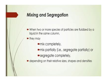
In that case, you will see that sometimes the liquid properties will affect the segregation and mixing inside the bed because, that gas has lower viscosity. Whereas, if you use the liquid then of course, there will be some difference in phenomena because of this a fluid properties.
