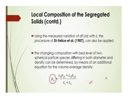
Now, using the measured variation of this frictional pressure gradient with height of the column, the procedure of this method a procedure of the that given by that Di Felice et al. 1987, can also be applied here by changing the composition with bed level up to a spherical particle species. And, that species will have of course, the different in both diameter and density.
