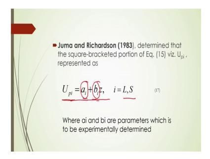
Now Juma and Rechardson 1983, they have also given another equations to calculate this that means, they are segregation velocity that is that along the axis of the fluidized bed and, they have given this equation of this here, U p i is equal to a i plus b i into z this a i and b i are the parameters which is to be experimentally determined, here I means L and S; that means, large and smaller particles.
