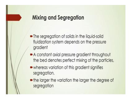
And, whereas the variation of this gradient of signifies there will be a segregation. And, the larger the variation pressure drop or pressure gradient larger the degree of segregation will be in the fluidized bed in case of liquid solid system.
