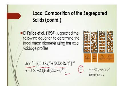
And, you will see their of course, to determine the local mean diameter using this axial voidage profile of course, during that complete or partial segregation the local voidage of the liquid there will be change at the top maybe higher voidage will be there whereas, at the bottom maybe lower voidage will be there.
