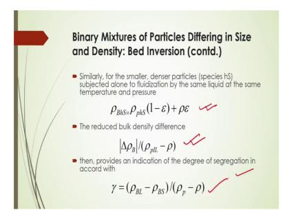
So, similarly for the smaller denser particles also you can expressed by this equation and, the reduced bulk density to be explained by this equation then, but it will provide the indication of the degree of segregation in accordance the to this equation here shown in the slides.
