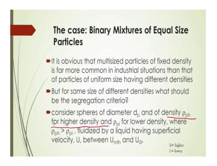
Now, some case let us see here for binary mixture of equal sized particles there, it is obvious that multi sized particles are fixed density is far more common, in industrial situation then that a particle of uniform size having different are densities of course, in different applications will not be having the same size of particles they are. For mixture of particles of course, there in that way that whenever you are making grinding and, then you not be having the same size particles there.
