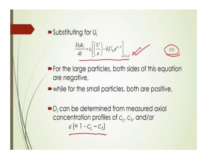
And substitution of this U i value here, you just a substitute it in equation number 13 there, then you will be a having this equation which is expressed by equation 15, they are and in this case for the large particles both sides of this equation are negative whereas, for the small particles both may be positive.
