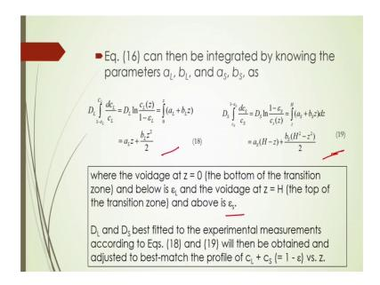
And from who is individually a for individual component of this larger and smaller particles are the dispersion coefficient you will be able to calculate. Here it is important that where, the voidage at z is equal to 0 the bottom part of the transition zone and below is the epsilon L and the voidage at that is at the top of the transition zone and above is epsilon S.
