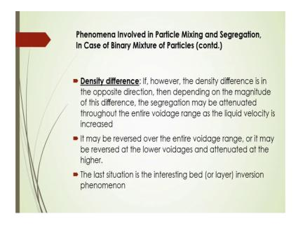
And, phenomena that involved in particle mixing and segregation that also depends on that density difference of that fluid particle, and also the voidage inside the bed or the density differences in the opposite direction then depending on the magnitude of this difference, the segregation may be may be attenuated a throughout the entire voidage range, as the liquid velocity is increased.
