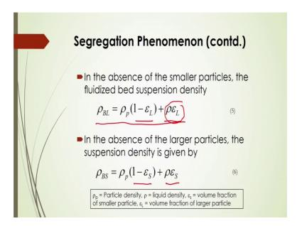
And, in the absence of smaller particles, so the fluidized bed suspension density to be actually calculated based on this equation 5 here.
