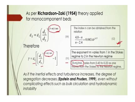
As per Richardson-Zaki 1954 they have developed one correlations for this gamma, which is applied for the monocomponent beds here. So, they have given this here gamma is equal to epsilon L into d L by d S to the power three minus m by m n. Where, this m and m n are the parameters, so that depends on the other properties of the fluid.
