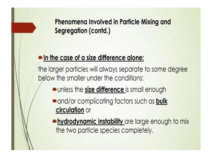
Now, what will be the phenomena involved in particle mixing and segregation there. In the case, of a size difference alone the larger particles will always a separate to some degree below the smaller under these following conditions there. So, their size difference one condition and so, bulk circulation or hydrodynamic instability. So, the larger particle separate to some degree below the smaller, unless the size difference is small enough.
