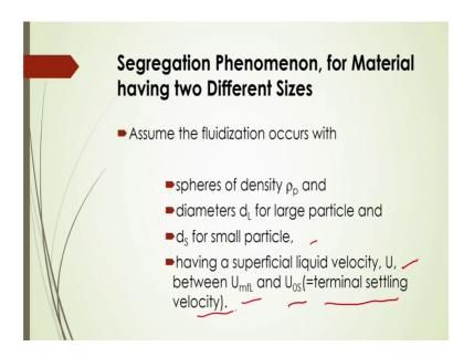
Now, how this segregation of phenomena for material having two different sizes can be obtained and can be actually quantified then. Let us, consider the fluidization that occurs with that spheres of density rho p and the diameters d L for large particles, and the diameter d S for the small particles. And, and having a spherical liquid velocity U they are between U m f L and U 0 S. U 0 S called terminal settling velocity for the particle of smaller size.
