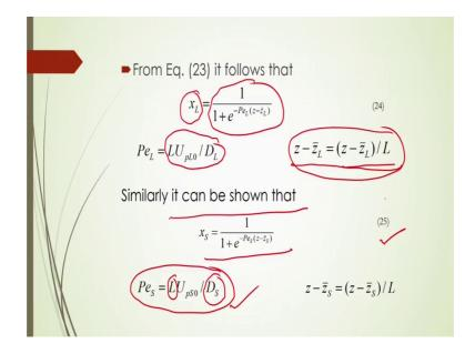
Now, from equation number 23 follows also that x L should be is equal to this here, we are this it will be related to this peclet number here, this peclet number is denoted by that axial dispersion coefficient of these large particles they are. So, if you know that axial dispersion coefficient of the large particles then you will be able to calculate what should be the mass flexion of the larger particles there in the bed.
