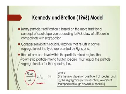
And, another important that, axial dispersion coefficient for this particle segregation will be there, then how this dispersion of the particles will be inside the bed Kennedy and Bretton 1966, they have actually interpret this phenomena that if binary particle stratification is in the fluidized bed, then based on this stratification axial dispersion according to the Fick's law of diffusion, in competition with the segregation can be explained.
