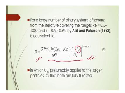
For a large number of binary systems of spheres from the literature covering, the range of Reynolds number that is 0.5 to 1000 and porosity of 0.50 to 0.95 Asif and Petersen 1993, they have suggested these correlations for this, dispersion coefficient of these larger or smaller particles inside the bed for their segregation phenomena.
