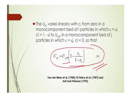
Now the U p i varies linearly with C i from 0 in a mono component made up for that i particles in which that epsilon will be is equal to epsilon i and C i will be equal to 1 minus epsilon i to U p i 0 in a mono component bed of z particles in which, you can say that epsilon is equal to epsilon j and C i will be equals to 0. So, that that U p i should be is equal to U p i 0 into 1 minus c i by 1 minus epsilon i.
