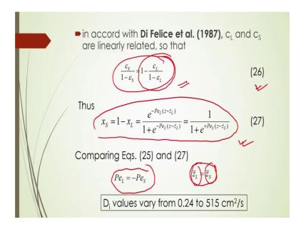
Now, Di Felice et al 1987, they have also are correlated with this C S and C L by they are what is that a porosity of the smaller and larger particles by equation number 26. And if you substitute this c S from this equation number 26, then x S can be calculated in terms of x L they are by this equation number 27. So, this is equation 27 actually is coming after simplification by substituting this concentration profile for the smaller particles in terms of larger particles.
