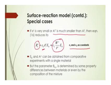
So, in that case, this equation 16; equation 16 will reduce to here this R t c that will be is equal to here c 2 into w c by r bar c into E b here c 1 and c 2 are here constants and this E b and sc can be obtained from that comparative experiments with a single material, but the parameter B sc which will be determined by some property difference between the material and a by the composition of the mixture.
