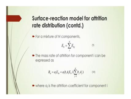
Also for a mixer of n components, what should be that energy breaking energy effective breaking energy associate with the component for that i and for that mixer.
