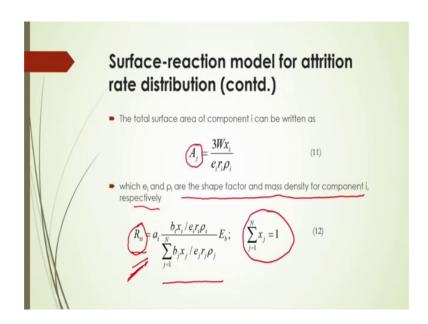
Now, the total surface area of the component i can be written as this A j, here total surface area of component i that is formed after attrition that will be is equal to what that W x i divided by e i r i rho i what is that e i? E i is the e i and rho i are the shape factor and mass density of the component i respectively.
