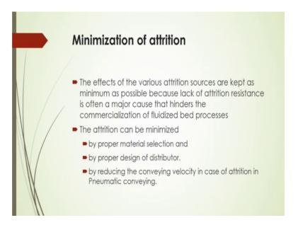
Another important that you have to choose the material a properly so, that the attrition should be less and you have to choose the material in such a way that, that material properties will not be changing significantly with the pressure and temperature.
