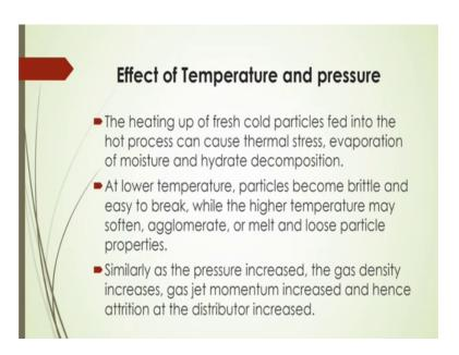
And the heating up of a fresh cold particles, you will see that is fed into the hot process can cause thermal stress. Now evaporation of moisture and the hydrate decomposition that is why the material properties physical properties will automatically change, there at lower temperature particles become brittle and easy to break while the higher temperature may soften agglomerate or melt and lose the particle properties.
