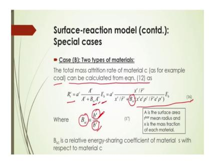
Now, surface reaction model; if we used for two types of materials suppose there is a mixture of coal and sand.
