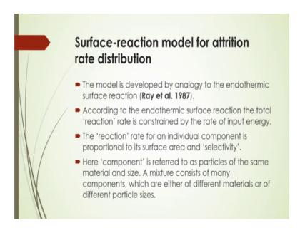
Now, surface reaction model for attrition rate distribution, the model, this actually developed by the analogy to the endothermic surface reaction which is given by Ray et al 1987. Now according to their model, they actually considered that there is some endothermic surface reaction a surface reaction and according to that reaction the total reaction rate is constituted by the rate of input energy.
