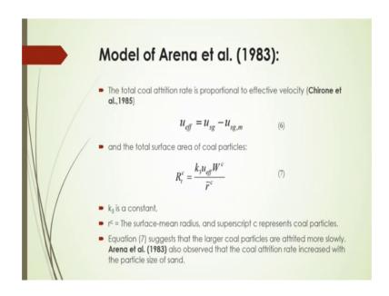
Here the total coal attrition rate there actually they have done this experiment with the coal particle. So, they have expressed into that the total coal attrition rate should be proportional to the effective velocity, there, what should that what should be the effective velocity; that were effective velocity should be what should be the relative velocity of the gas or fluid to its minimum velocity for its minimum fluidization.
