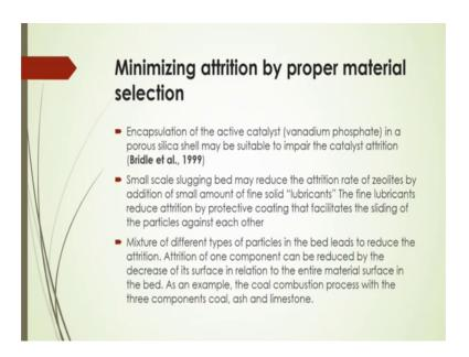
And encapsulation of the active catalyst like vanadium phosphate in a porous silica shell should be suitable to impair the catalyst attrition as per Bridle et al, 1999 and also it is seen that small scale slugging bed may reduce the attrition rate of zeolites by addition of small amount of fine solids that is called lubricants, if you use lubricants, there may be attrition rate should be a less because of surfaces smoothness the fine lubricants reduce
