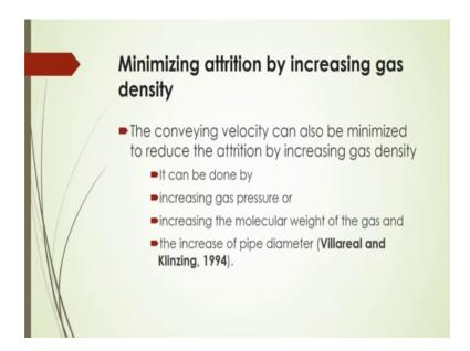
And if you increase that gas density; what will happen? Sometimes, it will minimize the attrition rate because they are gas density, it will of course, give the energy reduction and increase the gas pressure, who is increase the molecular weight of the gas and increase the pipe diameter which will effectively together will minimize this attrition rate; that is divide given by a Villareal and Klinzing, 1994 in their experiment.
