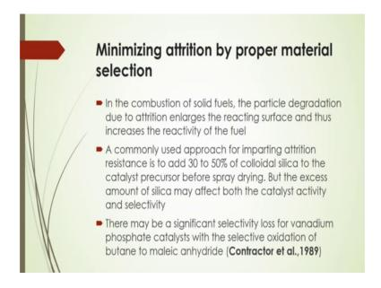
So, in that case, you have to use those materials let us see some example here the in the combustion of solid fuels the particle degradation due to the attrition enlarges the
