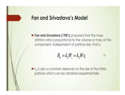
And Srivastava's model; as per their model, they proposed that the mass attrition rate should be proportional to the volume or mass of the component which will be independent of particle size.
