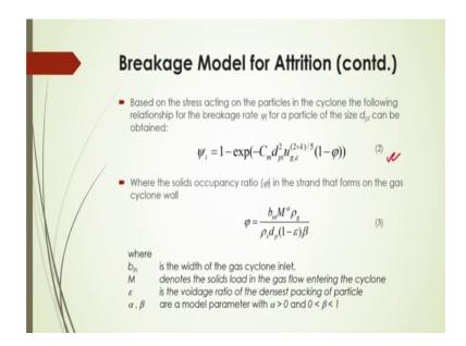
So, this is basically as per that Weichert model that these this breakage rate for particular class of particles, whether, it is coarser or finer that denoted by that class of the particles and it will be as i; the i means ith class here and the diameter of that particle in that particular classes it is denoted by d p i and for those class particles, what should be the stress and based on that is stress this breakage rate will be expressed as a psi i i for that class of particles here.
