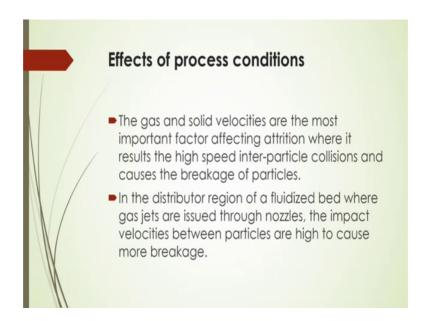
That also effect the attrition degree of attrition. Now in this case, you will see that higher speed maybe higher speed of the gas or higher velocity of the solid and gas may speed up the inter particle collisions and also the collision with the walls that may cause the more breakage of the particles into finer one.
