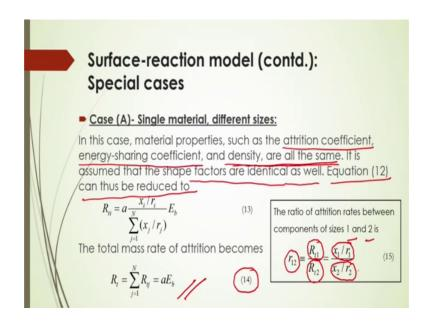
Now, for special cases, let us see the single material for different sizes. Now, in this case, material properties such as the attrition coefficient energy sharing coefficient and density are all same here. So, material properties, you have to take the material where attrition coefficient energy sharing coefficient that is b and then density for all for those material that will be same. So, it is assumed that the shape factors are identical as well also.
