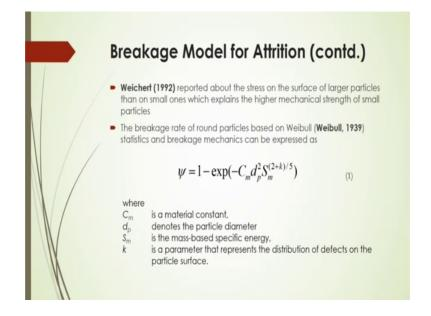
Now, Welchert 1992, actually stated that the stress on the surface of the large particles, then on small ones explains the higher mechanical strength of smaller particles and the breakage rate of round particles that based on the Weibull statistical analysis and breakage mechanics and that more rate because can be expressed based on that statistics and breakage mechanics by this equation 1.
