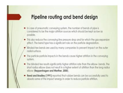
The in case of pneumatic conveying system; the number of bends of pipe is considered to be the measure attrition source which should be kept as low as possible there.
