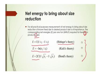
Now, net energy to bring about the size reduction what should be the net energy that is to reduce the size of the particle inside the bed. So, for all practical purposes, you can say this measurement of the net energy to bring about this reduction of this sides of the particles to the desired product size that is very crucial to know, here the corresponding net energies per unit of or you can say per unit ton required for the feed x 1 to the product x 2 here.
