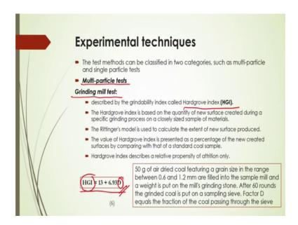
Now, experimental how to obtain this extent of this attrition here; so, the test methods can be classified into categories such as multi particle and then single particle tests here.
