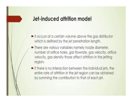
That a certain volume above the gas distributor which is defined by the jet penetration link and there are various variables of course, namely nozzle diameter number of orifice holes, even gas flow rate and then gas velocity orifice velocity gas density and all other parameters, sometimes, you will see that even size of the particles also the affect the attrition in the jetting region.
