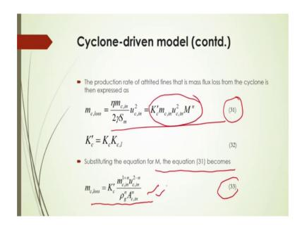
And also cyclone driven model as per that what should be the loss of fines from the cyclones that can be calculated from this equation here given as 31 eta m c in by 2 gamma into S m uc in square. So, this will be basically depending on the cyclone velocity and the mass of the fines that is collected here and substituting the equation for m; the equation 31, can be simplified and can be expressed by this equation 33 here.
