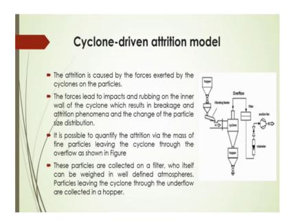
And cyclone driven attrition in this case, it is the actually happened because of the forces that exerted by the cyclones on the particles and the forces lead to impacts and rubbing on the inner wall of the cyclones which results in breakage and attrition phenomena and the change of the particle size distribution.
