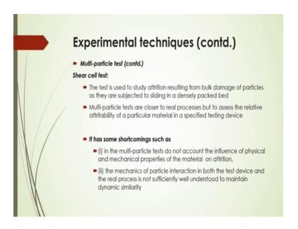
As per shear cell test, this test is used to study the attrition resulting from bulk change of particles as they are subjected to sliding in a closely packed bed there and multi particle tests are closer to the real process, but to assess the assess the a relative relative you can say attri tability of a particular material in a specified testing device.
