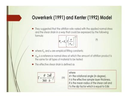
And Ouwerkerk 1991 and Kenter 1992 model; as per their model, they suggested that the attrition rate; that will be vary with the applied normal stress and the shear strain in a way that could be expressed by the following formula here.
