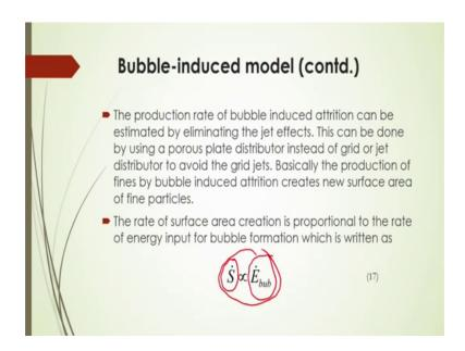
And the production rate of the bubble induced attrition can be actually obtained by eliminating the jet effects of course, and this can be obtained by using the porous play distributor for a distributor of a instead of grid or jet distributor to avoid the grid, grid jets, basically, the a production of the fines by bubble induced attrition that creates new surface area of fine particles.
