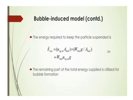
And the energy required to keep this particle suspended of course, is that is E suspension that will be is equal to u sg m into a bed and then here this m power your minimum fluidization a condition and then this W bed into g by a bed that will be is equal to W bed u sg m g. So, this is the energy required to keep the particle just suspended.
