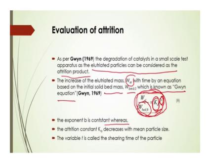
So, as per Gwyn 1969 that the degradation of the catalyst in a small scale tests apparatus, they have done as they are actually observation the elutriated particles can be considered as the attrition product and the increase of the elutriated mass that is W el with time by an equation based on the initial solid based mass that is W bed 0 which is known as Gwyn equation here.
