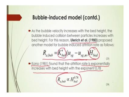
The bubble velocity increases, of course, the bubble induced collision between the particles, of course, will be increases with a bed height and for this region Ulerich at al 1980 proposed another model for bubble induced attrition rate as per here given in equation 23 or above that will be is equal to K dash bub into u sg minus u sg m into H bed here.
