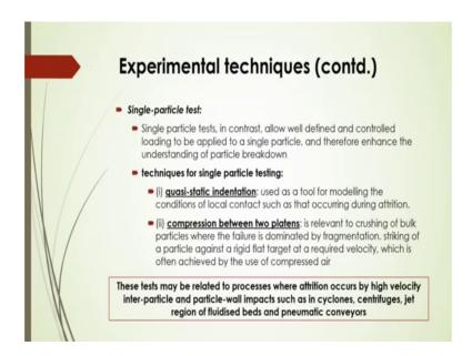
Single particle test in contrast, you can say allow well defined and controlled loading to be applied to a single particle there and therefore, you can say that entrance ah or you can say that the understanding of the particle breakdown is very easier by this single particle test.
