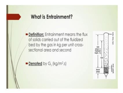
Now, before going to that first of all we have to know; what is that entrainment. Now as a definition you can say that the entrainment means the flux of solids that is being carried out the fluidized bed by the gas in k g per unit cross sectional area and second; that means, per unit time how much solids per unit cross sectional area will be actually carried out by the gas that is called entrainment.
