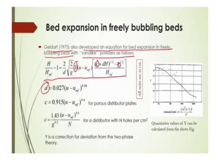
And also bed expansion if there is no coalesce or there is no breakup; that means, called freely bubbling beds in that case Geldart 1975 developed an equation for bed expansion in freely bubbling beds with sandlike powders as follows here like this.
