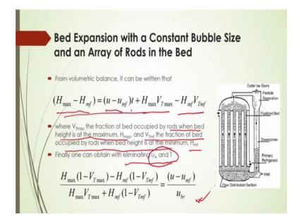
Now, bed expansion of course, it will be changing if you are just disturbed; if you are disturbing this fluid movement inside the bed by means of any mechanical device.
