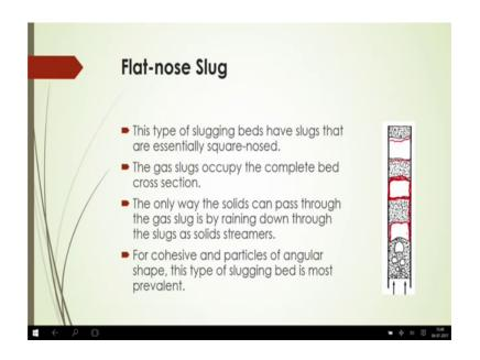
Whereas, flat nose slug this type of slugging bed have slugs that are essentially square nosed and the gas slug occupy the complete bed cross section. And the only way the solids can pass through the gas slug is by raining down through the slugs as solids streamers. For cohesive and particles of angular shape this type of slugging is most prevalent.
