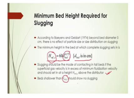
Now, what should be the minimum bed height required for this slugging of course, at any height you cannot get this slugging condition.
