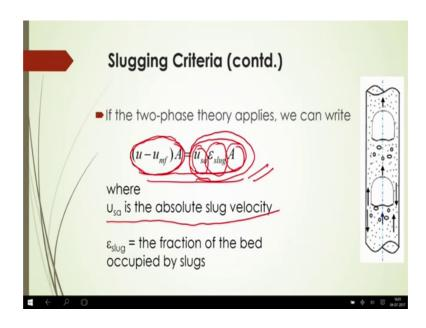
Another important criteria that is given by the that means Davidson; Stewart and Davidson; there they told that if the two phase theory applies then it can be written u minus u m f; that means, relative velocity of the based on the minimum fluidization velocity. And upon which you multiply by cross sectional area then what should be the total volume of the gas supplied to the bed and which will be equals to the volume of the
