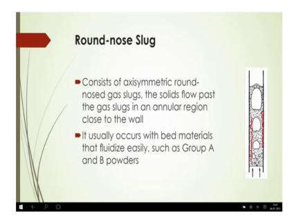
And here in this case a round shape or round nose slug that consists of axi symmetric round nosed gas slugs. The solids flow past the past the gas slugs in an annular region that is close to the wall. And it usually occurs with bed materials that fluidize easily such as like group A or group B particles as per that Geldart classification.
