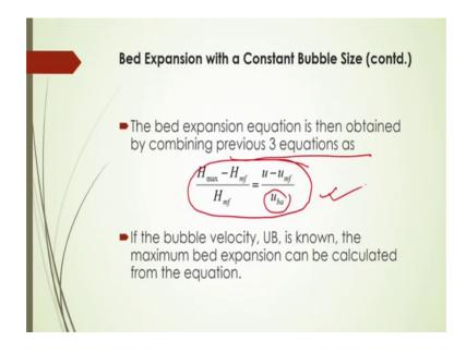
And the bed expansion equation is then obtained by combining previous three equations as this. So, this is the criteria for getting this maximum height of the bed.
