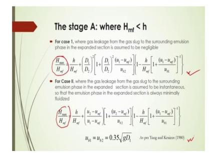
And then this the stage A where H m f is less than h; then you will be able to calculate this H max from this equation that is given in this graph. And also for case 2; that H max also to be calculated from this equation as per Yang and Keairns 1980.
