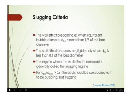
And what should be the then criteria for slugging that is very important when we can get the slugging phenomenon out of that bubbling fluidized bed. So, we are getting bubbling fluidized different types of bubbling fluidized bed of course, that is bubbling and past circulation and also that that is chant turbulent and they are also and then slugging fluidized bed; that is as a bubbling fluidized bed part of the bubbling fluidizing bed.
