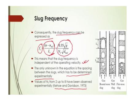
Another important point is that how many slugs will be formed inside the bed for a particular operation of the slugging condition. Now the slug frequency that is can be calculated of (Refer Time: 40:24) is denoted by f s to be calculated in this way that is u minus u m f by L S.
