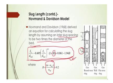
Now, Hovmand and Davidson 1968; they have derived an equation for calculating the slug length by assuming and inter slug spacing to be two times the diameter of the bed. They have taken a straight forward that bed number of beds is equal to 2 here.
