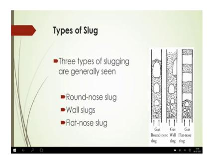
And here based on the fluid based on the flow rate of course, this slugging phenomenon will be there and there will be a different types of slugging that formed in the fluidized bed.
