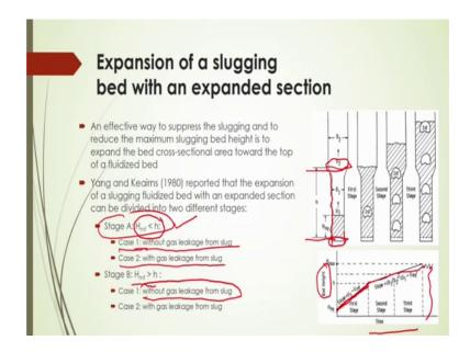
Expansion of the slugging of course, this expansion bed ah; if your slugging fluidized bed is expanding with the certain section then the effective way of suppression of the slugging and to reduce the maximum slugging bed height that can be of course, obtained from this minimum condition of this height.
