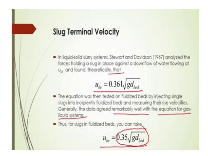
And then what should be the terminal velocity of the slug? We have already came to know that what should be the terminal velocity of the bubble for a particular its diameter. And what should be the bubble rise velocity when there will be only single bubble rises.
