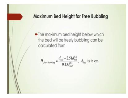
And what should be the maximum bed height? The maximum bed height below which the bed will be freely bubbling can be calculated from this correlations is given here.
