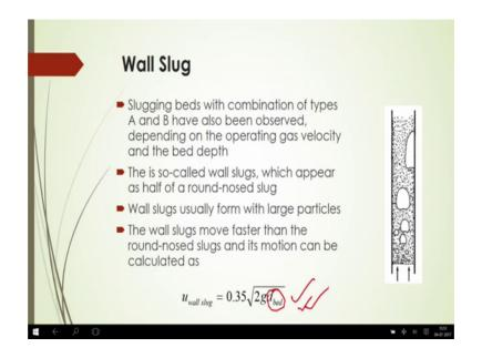
Whereas wall slug in this case you will see the slugging beds with combination of types A and B have also been observed. So, depending on the gas velocity and the bed depth this type of phenomenon will be observed.
