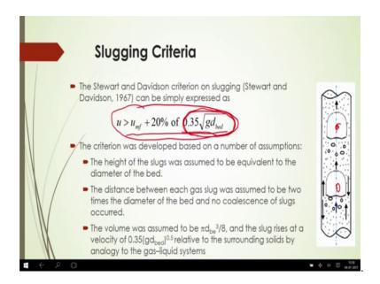
So, this is one important criteria when you can get the slugging phenomenon inside the bed. And the criterion was developed based on some assumptions; so in that case their assumption was there that the height of the slug that they have assumed that is to be equivalent to the diameter of the bed.
