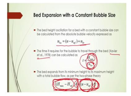
Again the bed expansion with a constant bubble size it is seen that that the bed height oscillation for a bed with a constant bubble size can be calculated from the absolute bubble rise velocity. Here this absolute bubble rise velocity will be is equal to u minus u m f plus u b r. The time it requires the bubble to travel through the bed that is as per Xavier et al 1978 can be calculated as this.
