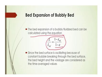
Bed expansion of bubbly bed; here the bed expansion of the bubbly the fluidized bed can be calculated using this equation from the ah; that means, material balance here L by L m f will be is equal to 1 minus epsilon m f by 1 minus epsilon. Since the bed surface is oscillating if any way because of constant bubble breaking through the bed surface, the bed height and the voidage are considered as the time averaged values here; this is very important.
