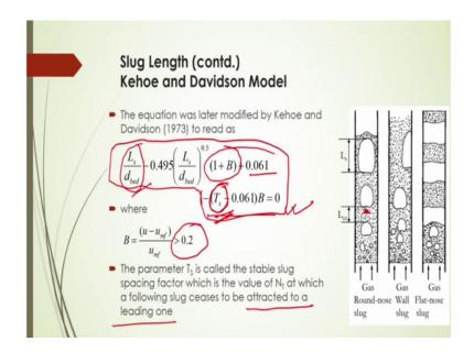
And the equation was later modified by Kehoe and Davidson 1973 to read as here in this case L S by d bed; that means, slug length to the bed diameter ratio minus 0.495 into L S by bed to the power 0.5 and into 1 minus into 1 plus B plus 0.061 minus this T S minus 0.061 into B that will be equals to 0.
