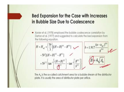
And then bed expansion for the case which increases in bubble size due to the coalescence. If there is a coalescence of bubble inside the bed and then bed expansion of course, will be changing in that case Xavier et al 1978 employed the bubble coalescence correlation by Darton et al 1977 and suggested to calculate the bed expansion from the following equation here.
