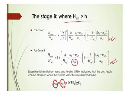
If the stage where H m f is greater than h then you have to use this equation to calculate the H max or; that means, maximum height and for case 2; it will be here.
