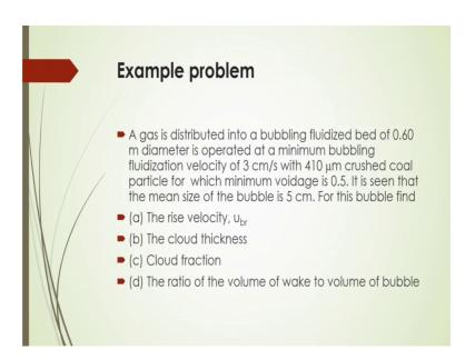
So, in this way we can calculate what should be the value of cloud fraction, what should be the this is cloud fraction is f c, and then what should be the ratio of volume of to the volume of bubble, that is f w and what should be the cloud thickness here.
