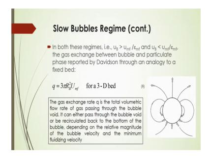
And also, in both these regimes, you will see if bubble rise velocity is greater than liquid velocity or fluid velocity, or that the bubble rise velocity is slower than the fluid velocity, there will be a there will be a gas change there will be a certain amount of gas, that will be change exchanged between bubble and particulate phase, that is reported by Davidson through a through an analogy to a fixed bed.
