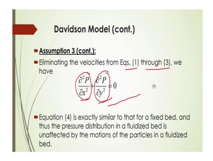
Again, this based on these the eliminating the velocity from the equation one through equation 3, we can get these, this in terms of this pressure what should be the continuity equation, and we can then express here this dou square or dou square P by dou x square plus, dou square P by dou y square is equal to 0.
