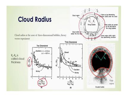
Cloud radius this cloud radius at the nose of 3-dimensional bubbles theory versus experiment it is shown here, this R c minus R B; that means, what will be the cloud radius what will be the bubble radius what will be the difference this R c minus R B is called cloud thickness.
