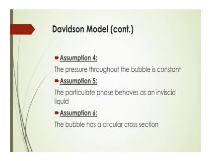
Now, other assumptions like here assumption 4, the pressure throughout the bubble is constant; that means, what will be the pressure surrounding the bubble, the through the bubble or through the bubble surface that will be constant, and assumption 5 the particulate phase that will behave as an in viscid liquid, there will be no viscose effect of the particulate phase that he has considered as in assumption 5.
