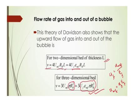
Now, what should be the flow rate of gas into an out of a bubble of course, whenever the bubbles will be moving as per that solid particles, since it is moving aside to the bubble and also into the bubble, and also cross over this bubble similar fashion of course, you will see the gas will also be moving, now that gas will be moving the upward motion, some gas will be coming into the that is bubble and also out of the bubble.
