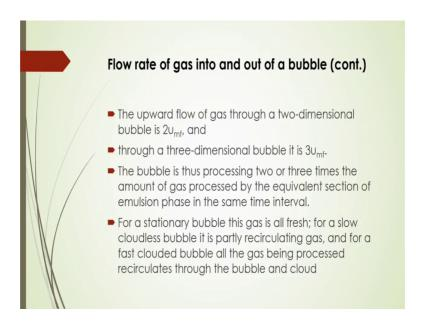
Flow rate of gas into and out of the bubble that of course, depends on that whether it is the 2-dimensional bed, or 3-dimensional bed and for 2-dimensional bed you will see that upward flow of gas through a 2-dimensional bed of course, it will be 2 times of minimum fluidization velocity.
