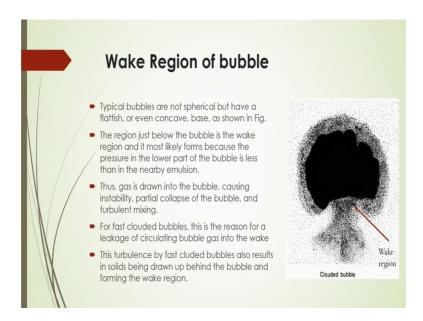
Here this wake region of the bubble, what that we have seen that bubble will whenever it will go up, it will carry some solid particles at it is wake region, and then what will be that wake region typical bubbles are not actually spherical at it is particular operation in the practical operation in this case, but have a flattish or even concave base as shown in the figure.
