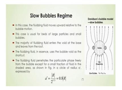
Now, you will see slow bubble regimes, in this case the fluidizing fluid moves upward relative to the bubble motion, and this case is usual for beds of large particles and small bubbles, and the majority of fluidizing bed, that enters the void at the base and leaves the roof here.
