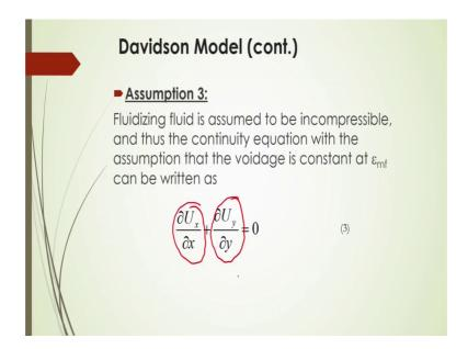
Now, as an assumption 3 the fluidizing fluid is assume to be incompressible here, and thus the continuity equation with the assumption that the voidage is constant at f silent m m, this minimum porosity of the fluidizing condition that can be retained as here, the summation of this relative velocity gradient in x and y direction that will be is equal to 0.
