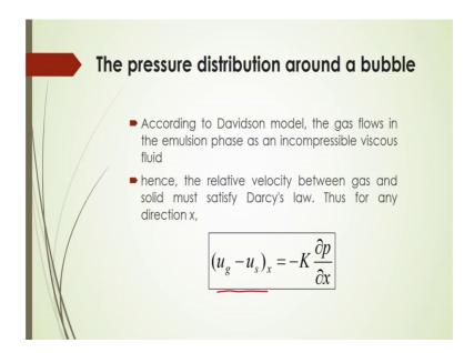
Now, that is what is the relative velocity of the solid particles relative to the fluid. Now, here u g minus u s means here gas velocity is the u s, u g and u s is the solid velocity, and that will be actually represented by this what will be the pressure gradient here.
