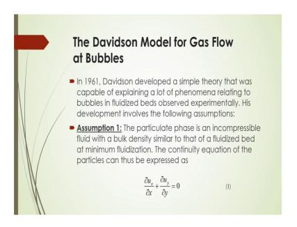
And here of course, we will see whenever solid particle will be moving surrounding the bubbles, there the solids will follow some pattern that is what should be the velocity or potential surrounding this bubble, and also what should be the pressure gradient surrounding the bubble, that depends on the bubble moving up or down based on the or according to the solid particle movement.
