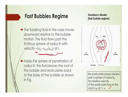
In this case moves downward related to the bubble motion, and the fluid flows past the fictitious sphere of radius R, with velocity that will be U b minus U m f by epsilon m f at r, here negative is because of this downward movement of the solid particles.
