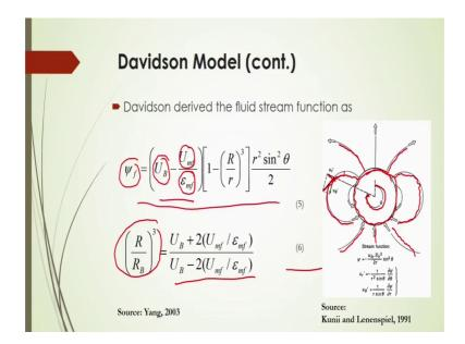
This fluid distribution function see the picture here this is one bubble, this bubble and surrounding this bubbles there will be a pressure gradient, and also the velocity of the gas, and also fluid you can say there will be some gradient kinetic energy distribution, because of this which the solid particle will here from this location will move aside and from the bottom solid particles will come to the bubble surface and.
