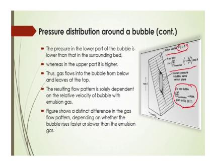
And then what should be that actual pressure distribution around a bubble, the pressure in the lower part of the bubble is lower than that in the surrounding bed here as per here figure it is shown.
