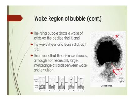
Now, wake region of course, you will see that depends on the size of the bubble, and also what will be rising velocity, the rising bubble drags a wake of solids up the bed behind it and the wake sheds and leaks a solid as it rises, this means that there is a continuous that is although not necessary in the large cases the interchanges of the solids between wake and emulsion. So, there will be a some interchange of the solid particles between wake and emulsion.
