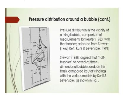
Here pressure distribution in the vicinity of a rising bubble, you will see in the figure comparison of the measurements by Reuter with the theories adopted from the Stewart, they have shown this phenomenon of the pressure distribution profile of the distribution surrounding the bubble.
