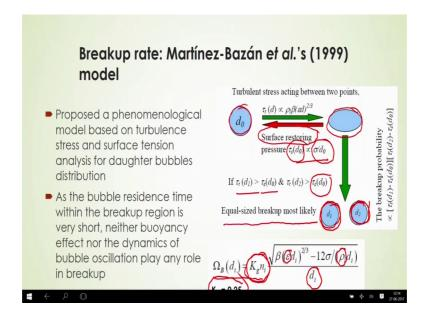
Martinez Bazan et als 1999 they have proposed a phenomenological model based on turbulence stress, and surface tension analysis for daughter bubble distribution, as the bubble residence time told within the breakup region is very short, neither buoyancy effect nor the dynamic of the bubble oscillation play any role in the breakup processes. So, in this case of course, this turbulence stress and the surface tensions, are very important factor for this breakup processes.
