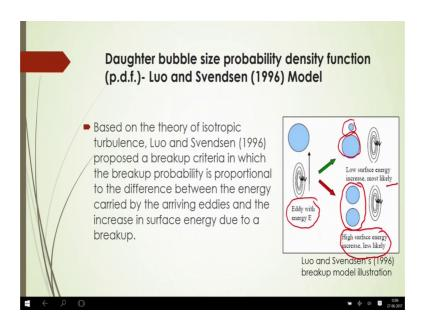
Now, daughter bubble size probability density function, how to calculate that after breaking up you will see that one bigger bubbles will form, number of a bubbles that bubbles that are form that may not be same as that that is source bubbles of course, and also that the size will be of course, different from that initial bubble, and those bubbles are formed after breaking those may not be the same may be same equal to each other.
