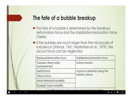
Now, what are the fate of a bubble breakup then, then the fate of a bubble is determined actually by the breakup or deformation force which is acting on this bubble and the stabilization or restoration forces of the bubble, now if the bubbles are much larger than the microscale of the turbulence, then you can say that the viscous force can be neglected. So, in that case there are different forces how it will be acting for this deformation of forces of course, we have to know.
