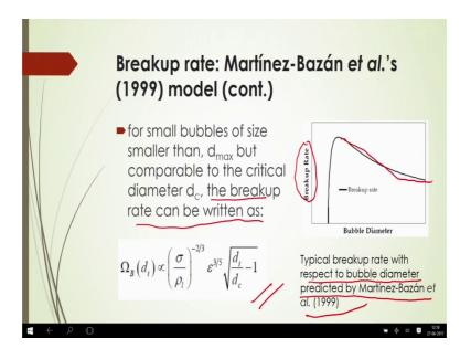
And for small bubbles of size if it is smaller than d max, but comparable to the critical diameter d c, then the breakup rate can be written as here by this equation, you can calculate the breakup rate from this equation now typical breakup rate with respect to the bubble diameter predicted y the Martinez Bazan et al 1999, they have given this bubble
