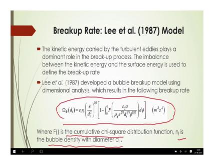
Now, this breakup rate as per this lee et al 1987 model, now as per this model this the kinetic energy is being carried out by the turbulent eddies which plays a dominant role in the breakup process, the imbalance between the kinetic energy and the surface energy actually will govern the breakup process, and this imbalance between this kinetic energy and the surface energy is cause to define the breakup rate.
