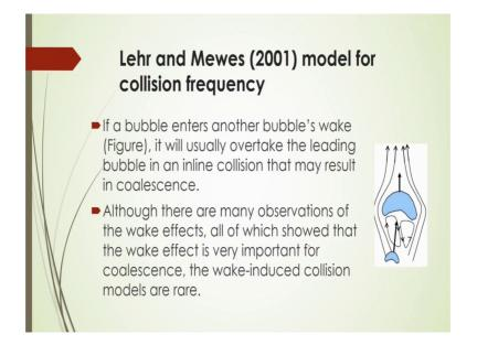
And if the bubble enters another bubbles wake according to the Lehr and Mewes, it will usually overtake leading bubble in an online in an inline collision that may result in coalescence and although there are many observations of the wake effects, all of which showed that the wake effect is very important for coalescence the wake induced collision models are very rare.
