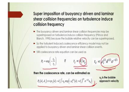
Now, another important that super imposition of buoyancy driven and laminar shear collision frequencies on turbulence induce collision frequency, the buoyancy driven and laminar shear collision frequencies may be superimposed on turbulence induce collision frequency as per prince and blanch 1990 and because the bubble relative velocity can be there superimposed. So, the turbulent induced coalescence efficiency model may not be applied to buoyancy driven and laminar shear collision models.
