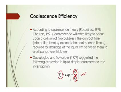
Now what should be the coalescence efficiency, then coalescence efficiency actually will be more likely to occur when the collision of 2 bubbles will be more intensive in that particular operation, if the contact time and the interaction time they are actually these 2 times are mainly governing this coalescence efficiency.
