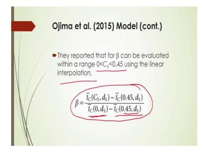
For beta can be evaluated within a range of particle concentration of this 0 to 0.45 using the linear interpolation like this here. So, this beta will be calculated from this equation here beta will be is equal to tc that is a function of Cs and ds minus tc bar that is what is that at particle concentration of 0.45 at the same particle diameter and also this tc 0 and ds.
