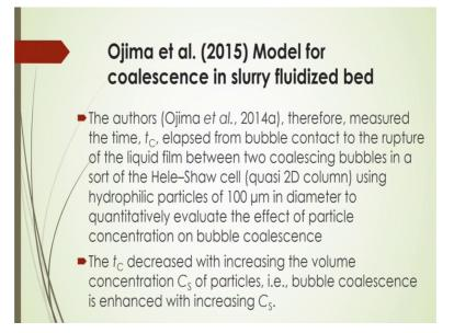
Ojima et al 2015 they have also presented 1 coalescence model in the slurry fluidized bed. So, in that case according to that ojima et al that they actually measured the time of coalescence and also based on which they actually derived the model in the quasi 2d columns by their experiment and they have interpreted that coalescence frequency according to their experimental results.
