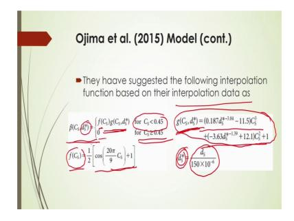
The following interpolation function based on their interpolation data as this beta C, beta is a function of that particle concentration and diameter of the particle, this diameter of this particle ds star is defined as this ds by 150 into 10 to the power minus 6. So, this is a again is a function of this concentration of the particle. So, it will be is equal to f as a function when the concentration is less than 0.45 and it will be 0 when the concentration is greater than equals to 0.45.
