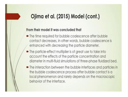
In other words bubbles coalescence is enhanced with decreasing the particle diameter, the particle effect multiplier is of great use in that case to take into account the effects of particle concentration and the diameter in multi fluid simulation of the 3 phase fluidized bed; the interaction between the bubble that depends on this concentration and also the particle size and governing equation of this bubble coalescence efficiency.
