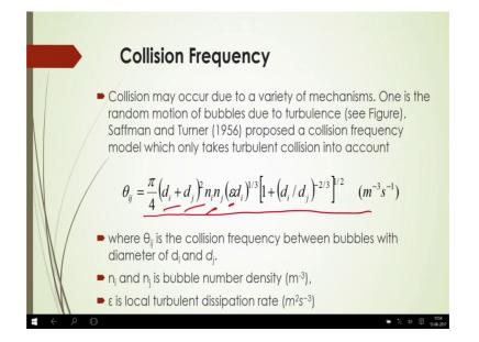
And then what is that collision frequency then you have to calculate first; what should be the collision frequency this collision may occur due to a variety of mechanisms, 1 is the random motion of the bubbles due to turbulence and in that case saffman and turner 1956 proposed a collision frequency model, which only takes turbulent collision into account.
