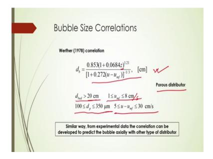
So, another correlations are 1978 Werther he has developed another correlations to predict the bubble size here for the porous distributor as d b is equal to 0.853 into 1 plus 0.0684 z to the power 1.21 by 1 plus 0.272 into u minus u mf to the power 1 by 3. From this correlations again you can calculate what should be the bubble diameter at a particular height jet.
