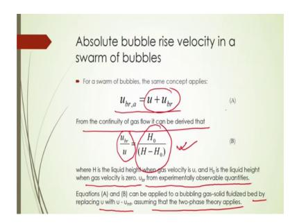
So, from the continuity of the gas flow it can be derived that this u br by u that will be is equal to H 0 by H minus H 0. What is this H? H is the liquid height when the gas velocity is u and H 0 is the liquid height when gas velocity is 0; and u br from the u br from experimentally observable quantities. So, this is very important in the liquid medium how to calculate the bubble rise velocity in a swarm of bubbles here.
