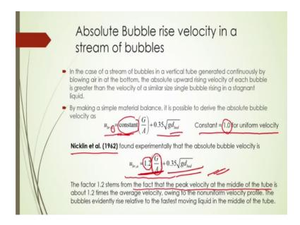
So, absolute bubble rise in a stream of bubbles then if there is more than one bubbles there will be interaction of bubbles and for which what should be the absolute bubble rise velocity.
