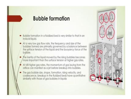
And you will see how then bubble is a formed inside this bubbling fluidized bed here see. The bubble formation in fluidized bed is very similar to that in an inviscid liquid of course, at a very low gas flow rate the frequency and size of the bubble formed primarily governed by the balance between the surface tension of the liquid are here in this case emulsion and the buoyancy force of the bubble.
