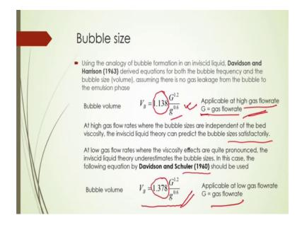
Now, what is this bubble size here? Using this analogous of bubble formation in an inviscid liquid Davidson and Harrison, 1963, derived equations for both the bubble frequency and the bubble size or you can say represented as volume here assuming there is no gas leakage from the bubble to emulsion phase.
