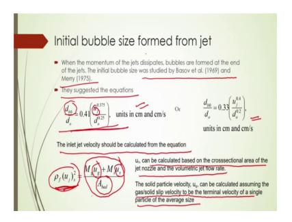
Now, initial bubble size that is formed from the jet when the momentum of the jet dissipated of course, bubbles are formed at the end of the jets. The initial bubble size was studied by Busov et al 1969 and Merry 1975 according to their proposed correlations you can calculate what should be the minimum, what should be the, what should be the initial bubble diameter that you can calculate from this correlations.
