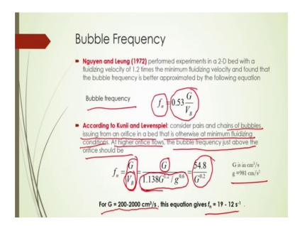
Now, bubble frequency what is that bubble frequency bubble frequency is the how many bubbles will be formed during this operation.
