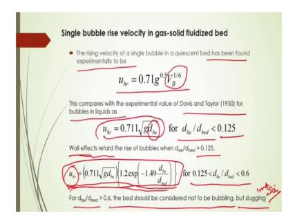
Now, single bubble rise velocity in a gas solid fluidized bed the rising velocity of a single bubble in a quiescent bed that has been found experimentally to be this 0.71 g to the power 0.5 into V B to the power 1 by 6. This is in terms of bubble volume. If you know the bubble volume what should be the bubble rise velocity. Of course, higher volume of the bubbles will have the higher diameter of course, equivalent diameter it will give you the more rise velocity.
