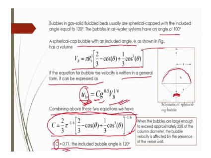
Now, bubbles in gas solid fluidized bed generally you will see different shape of bubbles are formed sometimes the spherical cap bubbles will form, and which may include the different angle which may be equal to 120 degree, the bubbles in air water system have an angle of 100 degree centigrade.
