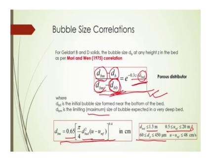
Now, to represent the bubble size or estimate or you can say predict the bubble size what should be the, actually how to estimate this bubble size. So, here Mori and Wen 1975 they have proposed one standard correlations to predict the bubble size which is depending on the axes of the bed from the distributor.
