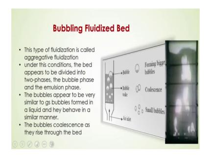
Now, what is bubbling fluidized bed? What is that fluidized bed? Already we have discussed in earlier lecture that how bubbles are forming inside the fluidized bed and what will be the characteristics of the bubbling fluidized bed.
