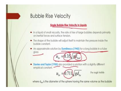
Now, what should be the bubble rise velocity? Once you know the bubble size and also once you know the bed effective bubble size or you can say the equivalent bubble diameter and also bed diameter, how to calculate the bubble rise velocity there.
