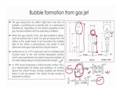
Now, how this bubble is formed from the gas jet let us see. The gas issuing from an orifice might be in the form of bubbles as a pulsating jets or periodic jet, or you can say a
