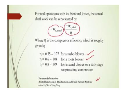
Now, for real operation then or practical operations then it is frictional losses we can say the actual shaft work can be represented by this W s actual that will be is equal to W s ideal divided by eta; eta is the efficiency of the compressor which is roughly given by this eta will be is equal to 0.55 to 0.75; that means, efficiency 55 percent to 75 percent for turbo-blower and it will be 60 percent to 80 percent if it is rooters blower.
