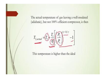
And then actual temperature of the gas leaving a well insulated adiabatic, but not 100 percent efficient compressor is then calculated by this T 2 actual will be is equal to T 1 plus T 1 by eta into P 2 by P 1 to the power gamma minus 1 gamma minus 1. So, what should be the actual temperature at it is higher temperature if you are considering that there will be a fictional losses during the operation of the compression from this lower pressure to the higher pressure.
