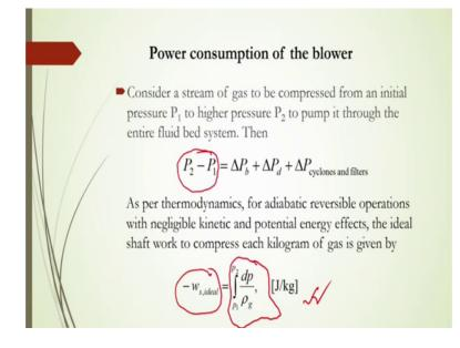
Now, power consumption of the blower let us see here how to calculate. In this case you will see that a stream of gas which will be compressed from an initial pressure to higher pressure if you consider that initial pressure is P 1 and the higher pressure is P 2 the then gas is to be compressed from this lower pressure of P 1 to the higher pressure P 2 to pump this gas through the entire fluid bed in the fluidized bed.
