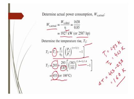
Then what should be then the actual power consumption if the if the compressor or blower efficiency is 85 percent then shaft work actual shaft work will be is equal to W s ideal by eta it has deficiency of the compressor then it will be 1683 divided by 0.85 then it is final is coming 1927 kilo watt or you expressed as 2587 horse power.
