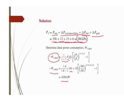
Here this solution what is this you have to calculate first what should be the what should be the pressure that is final pressure P 2 then final pressure P 2 will be is equal to what should be the P exit pressure. What should be the pressure contribution by the cyclones and filters what should be the bed pressure drop and what should be the distributor pressure drop which is as used as grid here.
