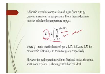
Now, adiabatic reversible compression of the gas from this lower pressure P 1 to the higher pressure that may cause an increase in temperature because of this pressure difference. Now from thermodynamics points of view of course, you one can calculate the temperature at P 2 as what should be the P 2 T 2 as this P 2 that means, if we compress this gas from this lower pressure to higher pressure at that higher pressure what should be the temperature change.
