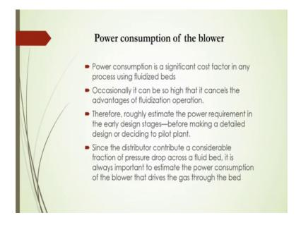
So, let us see how to calculate what should be the actual fiamble of this power consumption of the blower you will see that power consumption is a significant cost factor in any process using fluidized beds. Occasionally you will see it can be so high that it cancels the advantages of fluidization operation.
