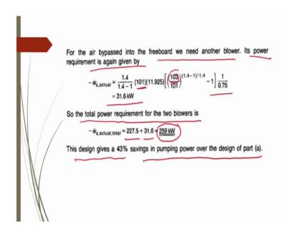
So, for the air bypassed into the freeboard we need another blower of course, or compressor it is blower requirement is again given by this again the same equation to be used to calculate the actual shaft work as this. So, it is coming here of course, this is function of pressure this is initial pressure, this is this pressure here it will be 103 because this at this region the atmospheric pressure is 103 kilopascal here.
