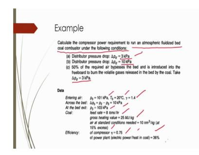
Now, let us see another example if we use the if we use the distributor in such way that it is the pressure drop is some value and if we if we distribute the gas in two locations or it will bypass this gas in such way different condition then what should be the power consumption.
