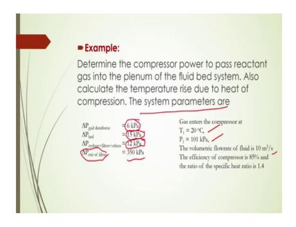
Now, let us see one example that how to calculate this pressure compressor power to calculate to calculate the power of gas distribution into the plenum of the fluidized bed system by this compressor by compressor or any blower, also calculate how to calculate the temperature rise due to the heat of compression here.
