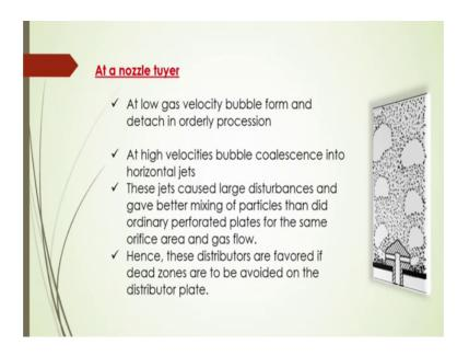
At a nozzle tuyer it is seen that, at low gas velocity bubbles form and detach in orderly procession like this here in this figure. At high velocities bubble coalescence into horizontal jets, these jets caused large disturbances and gave better mixing of particles and did ordinary perforated plates for the same orifice area and gas flow rate. Hence in this case these distributor are favored if dead zones are to be avoided on the distributor plate.
