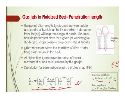
Gas jets in fluidize bed now penetration, penetration length what is that penetration length? The penetration length here what is that penetration length see in this figure, the from this gas jet at the top there will be permission of bubbles, and what is the center of this bubbles and from the entry point of this gas from the distributor, and this distance is called penetration length.
