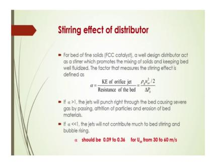
ah The factor that measures this stirring effect is defined as which is denoted by alpha which is nothing, but the ratio of kinetic energy of the orifice jet the resistance of the bed. This kinetic energy of the orifice jet is given a half of row g U o r square U o r is nothing, but the orifice velocity and resistance of the bed will be represented by the pressure drop of the bed.
