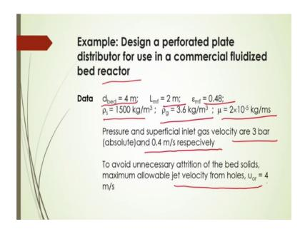
Let us see one example here like design of a perforated plate distributor for use in a commercial fluidized bed reactor. Now it is given that bed diameter is given minimum height of the fluidization is given, minimum porous it is given, density of the solid which is being used for that distributor is given to you, what will be the density of the gas is being used, what is the viscosity.
