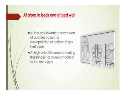
And then at pipes in beds and at bed wall this is at low gas flow rate a succession of bubbles occurs for down pointing or horizontal gas inlet pipes. At high velocities result standing flickering jet or plumb attached to the entry pipe like this in this figure and gas jets in fluidized bed. How gas jet is formed in this fluidized bed from the distributor.
