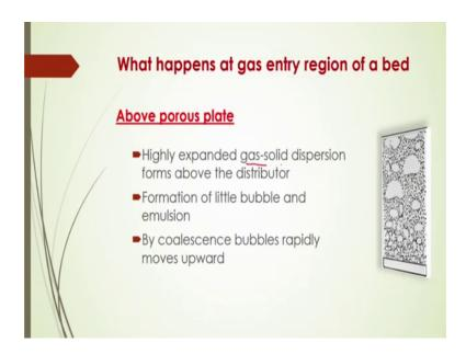
Now, what happens at gas entry region of a bed above porous plate? It is seen that highly expanded gas solid dispersion forms above the distributor, and also formation of little bubble and emulsion it is seen whenever gas is distributed from the porous plate and at its region of this distributor. By coalescence bubbles rapidly move upward due to their higher bounce above also perforated plate here.
