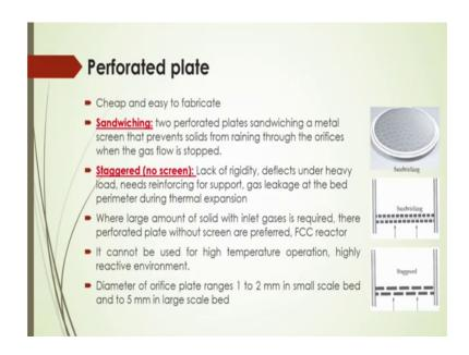
And here let us see, what is the characteristics of the perforated plate? So, this perforated plate see the figure here diagram or given here different types of perforated plates are also available commercially. So, these perforated plates are cheap and easy to fabricate, some perforated plates are sandwiching some perforated plates are staggered with screen and without screen.
