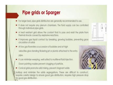
And another is called pipe grids or sparger. In this case if the picture here this is the one pipe through the pipe gas is coming and also in each saw pipe of this here, there will be a force and through which this bubbles are coming and gas is coming and permits a bubbles and it will be distributed inside the bed.
