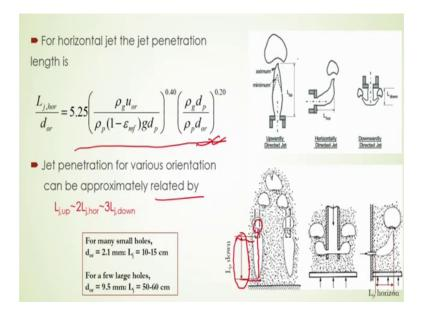
For horizontal jet the jet penetration length can be calculated from this relationship here, again this depends on this particle density minimum fluidization velocity even orifice velocity is there. So, from this correlation you can calculate what should be the penetration length if it is horizontally moving. So, and also there is a rough relationship
