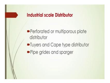
Now, what are those industrial scale distributor then we used for fluidized bed. Let us see again different types of industrial scale distributors are available, one is perforated or multiporous plate distributor. Some other that Tuyers or cape type distributor and some others are pipe grides and sparger. So, all those distributor have some advantage and some disadvantage of course, we will be discussing successively.
