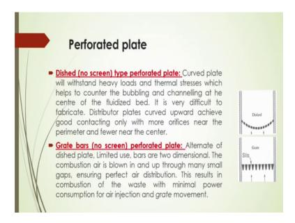
And other different type of perforated plates like dished type perforated plate; in this case it will be curve shape this curve shape dished perforated plate. In this case this type of perforated plate withstand heavy loads and thermal stresses, which helps to counter the bubbling and channeling at the center of the fluidized bed.
