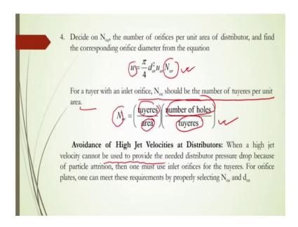
After that you have to decide how many holes of the orifice per unit area of the distributor to be maintained, and you have to find out the corresponding orifice diameter from the equation given here. For a tuyer with an inlet orifice N o r should be number of tuyers per unit area, should be calculated from this. This N word designed as what is the tuyers per unit area and number of holes for unit tuyers.
