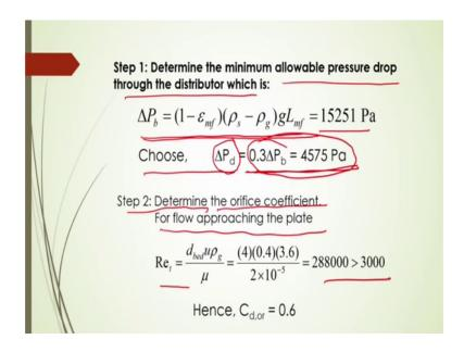
So, as per that procedure step 1 you have to determine what will be the minimum allowable pressure drop through the distributor, which can be calculated from this equation what should be the bed pressure here. This will be is equal to this thus after substitution of the data and then choose, what should be the delta P d. As per recommendation it should be 30 percent average of that 0.1 to 0.23.
