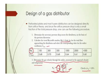
Now, design of a gas distributor, now how to design this gas let us see some step by step procedure here, let us see here perforated plates and most tuyer distributors can be designed directly from orifice theory and since the orifice pressure drop is only a small fraction of the total pressure drop, one can use this following procedure here.
