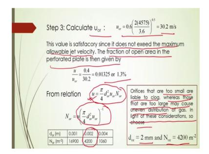
After that calculate U o r by that equation and then you are getting this and this value is satisfactory since it does not exceed the maximum allowable jet velocity, the fraction of open area in the perforated plate then given by this u by U o r from this 1.3 percent. So, from this equation of this you have to then find out what should be the number of orifice holes to be maintained here.
