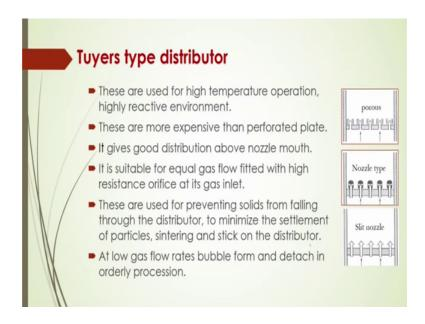
Another type is called Tuyer type distributor, these are generally used for high temperature operation and it is also it is suitable for highly reactive environment. These are more expensive for operation than perforated plate, it gives good distribution above the nozzle mouth and also it is suitable for equal gas flow through the distributor, and also if there is high resistance orifice are been used for this type of Tuyers, then you can evenly distribute the gas inside the bed.
