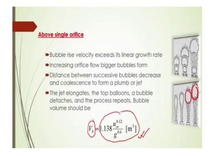
And increasing orifice flow bigger bubbles form. Distance between successive bubble decrease and coalescence to form a plump or jet. The jet elongates the top balloons a bubble detaches here this bubble here in this balloon you can say here bubbles will detaches and the process is repeated and bubble volume will be then bubble will then will go up and move with a certain velocity, and it will be dissolved.
