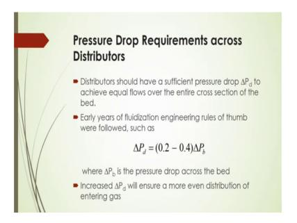
Now, what should be the pressure drop requirements across the distributors to get the uniform distribution of the gas through the distributor? And for this design of this distributor of course, you have to know the pressure drop requirements. This pressure drop of course, sufficient pressure drop should be there to achieve equal flows over the entire cross section of the bed.
