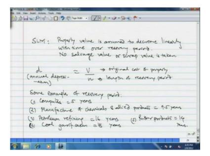
The simplest one is the straight line method S L M, here the property value is assumed to decrease linearly with time, over the recovery period or in that case more salvage value or scrap value is taken. So, then the depreciation angle depreciation d that, we denote is equal to v the original investment in property at start divided by n, where the length of straight line recovery period, v is the original investment in property or original cost of property and n is the length of recovery period.
