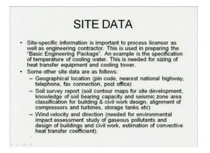
Then, we have to also gather some site data, site specific information is important to process licensor as well as the engineering contractor because this is used for preparation of the basic engineering package. An example is the specification of the temperature of cooling water, this is needed for sizing of the heat transfer equipment and also the cooling tower then unarise temperature, humidity, etcetera.
