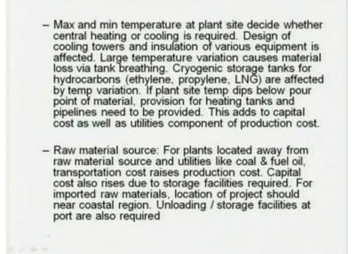
Then, the third one is the temperature, the minimum and maximum temperature at the plant site has a direct impact again on capital and operating cost. Design of cooling tower, air cooler or plant insulation is affected by temperature then the buildings for plant administrative purpose such as the worker amenities or control room may need to be air conditioned depending on the duration of hot period.
