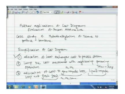
Now, how we can do that in that we introduced the concept of lumping of the cost, we have to we decided that we shall lump the cost. And then what we did we followed a 3 step strategy allocation of the heat exchanger cost to the process stream. Then lump the cost associated with the laboring process operation and allocation of the cost to 3 loops or 3 streams.
