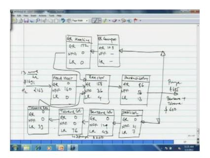
So, that we write 109 here, there is no net fresh feed neither liquid recycle. Now gas recycle heating, gas recycle heating if you go to the heating and cooling loads, you will find the gas recycle heating is 172 dollars here. So, that we put here the reactor is 198
