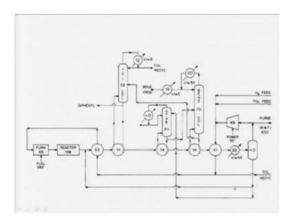
We start with the simple gas compression, gas compression as you will see in the flow sheet is the total cost is 109, because 49 1000 dollars for the compressor 60 1000 dollar for the power.
