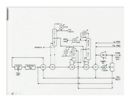
And then we identified 5 heat exchangers in the in the process that i just showed to you. The first heat exchanger that exchange a heat between reactor effluent and the recycle toluene. Then the toluene re boiler, then stabilizer re boiler, benzene re boiler then the fresh feed and reactor effluent heat exchanger and finally, the cooling the condenser.
