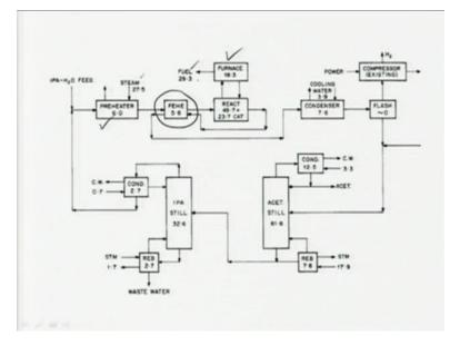
Similarly, we also saw the as how we can optimize the heat transfer in the process, for that flow sheet is now on the screen. Here you can see that the heat from the reactor effluent a stream emerging out of the reactor is recovered in the incoming stream. In the incoming stream through this f e h e feed to effluent heat exchanger and a feed to effluent heat exchanger is quite small as compared to the pre heater and the furnace, which supply heat to the feed that increases the cost of operation.
