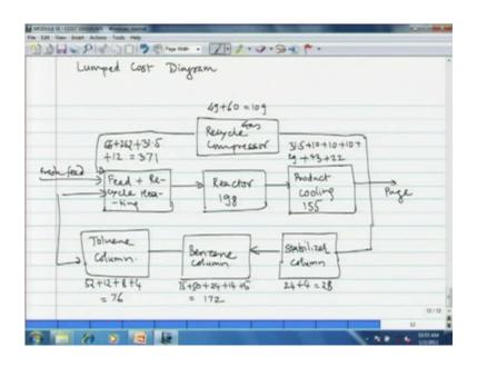
We have feed plus recycle heating, then the reactor then product cooling. Now from product cooling, we have the product as well as gas recycle purge streams emerging, the liquid is separated in 3 columns stabilizer benzene. Now this is our lumped cost diagram, where we have listed 7 major operations in the process. And we have connected them as how in the in the proper order, now let us gather the cost that is associated for each of these operations.
