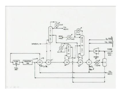
And then we saw the heat integrated flow sheet, but heat integrated flow sheet is rather complex, because of several exchangers that are there we saw that how the a reactor effluent was giving up it is heat to the feed. This is the recycle toluene then the re boiler of toluene column, re boiler of stabilizer column, re boiler of benzene column. Then it was also giving heat to the fresh feed that is coming in this hydrogen and toluene fresh feed.
