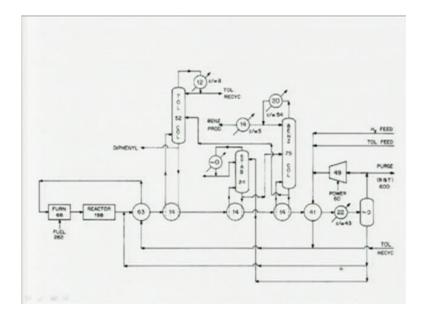
Now, reactor if you go to the main flow sheet, we see that a reactor annualized cost of the reactor is 198 1000 dollars. So, that we attached now here 198 1000 dollars. Now next the feed and recycle heating, let us go back to the flow sheet, we have here 2 heat exchangers that heat the feed fresh as well as recycle feed. And then we also have a furnace that does the job.
