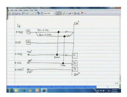
The bigger segment is matched with C 1 and sorry match with C 1 and heat load here is 8 megawatt. So, the segment of H 1 is now ticked off, okay? C 1 is already ticked off, now H 1 is completely ticked off. Now, we are left with one hot stream and one cold stream.
