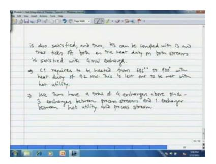
We thus have a total of four exchangers above pinch three exchangers, between process streams and one exchanger between cold utility sorry hot utility and process stream. So, that completes the design pinch design above or the pinch heat exchanger design above pinch.
