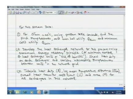
For this stream data we have to answer three questions; first is that for delta T mean equal to 20 degree centigrade, we have to find the minimum hot utility and minimum cold utility, as well as the pinch temperature using problem table cascade. Then the second question is the development of the heat exchanger network for the process using maximum energy recovery principle or minimum number of heat exchanger unit or what is known as tick off heuristic; that we have seen in the theory lectures.
