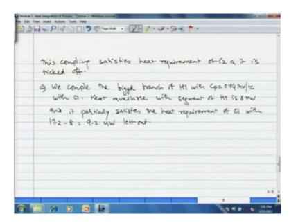
So, that point we note we couple the bigger branch of H 1 with C p of 0.04 megawatt per degree centigrade with C 1 heat available with segment of H 1 is 8 megawatt. It partially satisfies the heat requirement of C 1 with 17.2 minus 8; that is 9.2 megawatt left out, now we make the second match segment of H 1.
