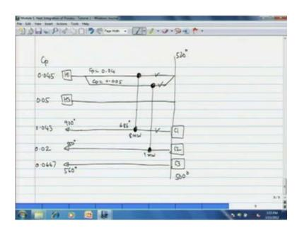
We write it here 686 degree centigrade, now we are left with one hot stream H 3 and second hot stream C 3 second cold stream C 3. Now, if you look at the heat capacity and the requirement H 3 has a heat capacity of 0.05, which is lesser that 0.0667. So, it can be easily coupled and the heat that is available with H 3 is exactly the requirement of C 3. Therefore, H 3 C, C 3 can be coupled that point.
