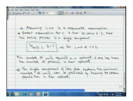
Assuming L to be 0 is the reasonable assumption because; in a process all of the points will be connected by one or the other way. So, the number of independent loops will be 0 as we saw in case of graph two as in case of loop components and the number of loops were. So, in process having many, many streams that coupled to each other assuming L equal to 0 is a reasonable assumption.
