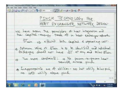
So, the pinch technology for heat exchanger network design. We have seen before the principal of energy integration of the system and then the capital energy trade off in the heat exchanger network.
