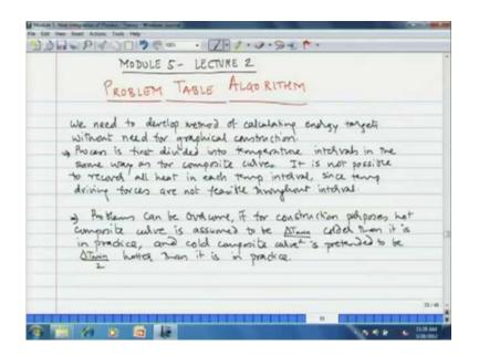
So, we shall now see an alternate algorithm for determination of minimum hot and cold utility of the process that is known as problem table algorithm. We need to develop method for calculate the energy targets without need for graphical construction. The process is first divided into the temperature intervals in the same way as for the complete curves, it is not possible to recover all heat in each temperature interval.
