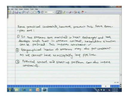
Now, there are certain process constraints ok. So far, we have assumed that any hot steam can mixed with any cold steam are can be coupled not mixed. It be coupled can be coupled with any cold steam provided there is no feasible temperature difference between the 2. But some practical constraints are available or possible; some practical constraints can prevent this particular coupling.
