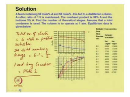
So, 1, 2, 3, 4, 5, 6 total number of plates is equal to 6 with a partial reboiler, the total number of total number of trays is equal to 6 minus 1 is equal to 5. And the optimum feed tray locations feed tray location is equal to we can see which is the saturated liquid which is over here, plate number two plate two this way we can obtain the number of ideal stages required, and locate the feed tray.
