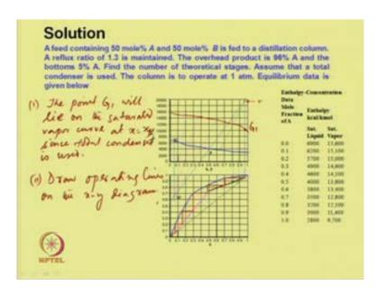
And then the point G 1 which is over here, G 1 will lie on the saturated vapor curve at x is equal to X D, since total condenser is used. Now, we can draw operating lines on the x, y diagram operating lines are drawn between these two sections, and then the contraction was followed from this points over here.
