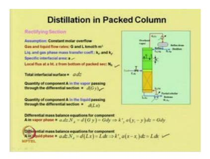
Let us considered the rectifying section how to do the balance, for the rectifying section we have following assumptions constant molar over flow, liquid and gas flow rate G and L respectively, liquid and gas phase mass transfer co-efficient small k, x dash and k, y dash, specific interfacial area A. And local flax at a particular height Z from the bottom of the packed section is N A, now total interfacial surface would be a d z, so we have taken a essential section of thickness d z.
