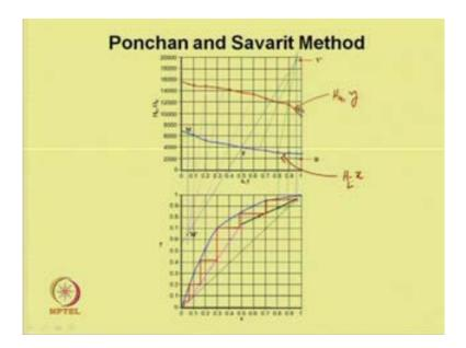
In this case we know the equilibrium data, x, y data and we know the H enthalpy of the liquid, and enthalpy of the vapor. And so we can plot the lower curve represents, H L x and this is H G y.
