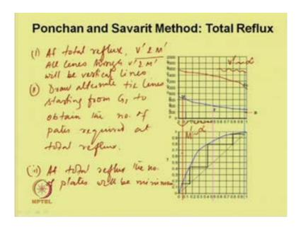
Now, we will discuss the total reflux, at total reflux total reflux the point V dash and M dash this two points will be add infinity (No audio from 16:54 to 17:10), this two points will be M dash and V dash will be at infinity, the line which will joint between M dash and V dash will be a vertical line. So, all the lines between M dash and V dash will be the vertical line, so V dash and M dash will be vertical lines.
