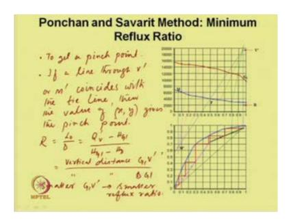
Now, using Ponchon and Savarit method, we could obtain the minimum reflux ratio to obtain the minimum reflux ratio which is R mean, we need to obtain the pinch point, first to get a pinch point to obtain the pinch point if a line through V dash or M dash coincides
