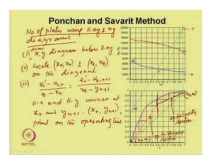
Now, let us see how to obtain the number of plates using H x, y and x, y diagram. So, first we have to draw the x, y diagram below H x, y diagram with the similar scale, and then locate x w, x w and x D, x D on the diagonal, which is located over here, and another point is located over here. So, on the diagram the point x w, x w and x D, x D, so this points are located and then as we know from the earlier derivations Q v dash minus
