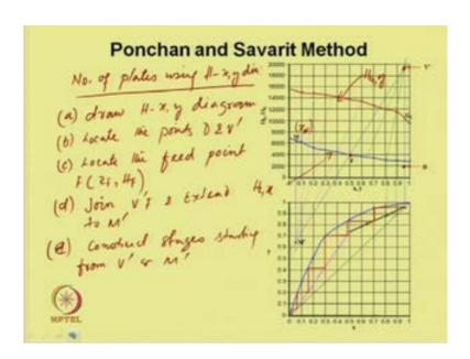
First we will consider number of plates, number of plates using H x, y diagram here, first we have to draw H x, y diagram with the help of given data which is plotted over here,
