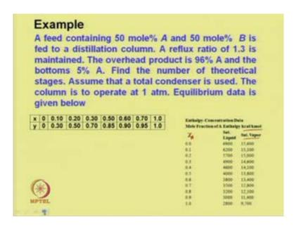
Let us take an example for calculations of the number of plates, using Ponchon-Savarit method a feet containing 50 mole percent A, and 50 mole percent B a feat to a distillation column. A reflux ratio of 1.3 each maintains the over head product is 96 percent A, and the bottom is 5 percent A, find the number of theoretical stages. Assume that a total condenser is use, the column is to operate at one atmosphere equilibrium data
