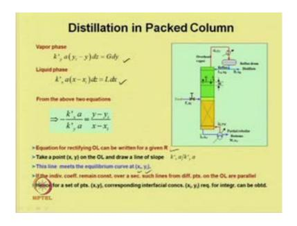
Now, how to get this interfacial concentration for a set of values of y, if we considered the vapor phase and the liquid phase this two relation, and if we divide this two equitation the ratio of mass transfer co efficient. We know the equation of operating line for a rectifying section for a given R, and we can take a point x, y on the operating and line draw a line of the slope of a x dash a divided by k y dash a.
