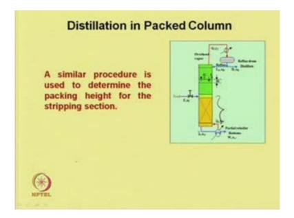
A similar procedure is used to determine the packing height for the stripping section. So, far we have discussed the design procedure, how to obtain the packing height in the rectifying section, similar procedure should be adopted to obtain the height of packing in the stripping section. So, that the total height required for a given separation can be obtained.
