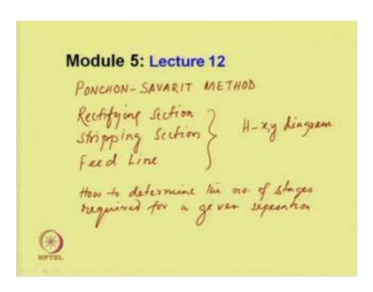
Let us have a recap of our previous lecture on this topic; in our previous lecture we have primarily considered the design of a distillation column, by Ponchon and Savarit method, Ponchon-Savarit method. Primarily we have discussed for a fractionators, what is the balance equations for the rectifying section section, stripping section and feed line. All the balance equations we have derived. And we know how to construct the H x, y diagram; that is enthalpy concentration diagram.
