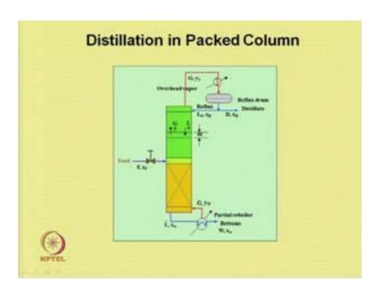
Now, we will discuss height and number of transfer unit method, this is typical pack distillation column, where feed enters at particular locations with a composition Z F. And we have reflux dram, and the distillate there is a condenser and similarly, at the bottom we have partial reboiler as in distillation.
