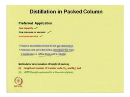
Now, we will discuss distillation in packed column, in some cases where packed column distillation is vapor, particularly in case of low capacity applications or low pressure or
