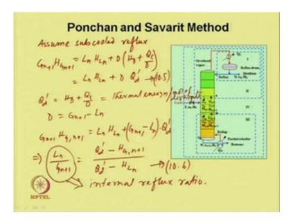
If we assume the reflux which is coming out it may be sub cooled reflux. Assume sub cooled reflux and the mol fractions is x D for 8 then we can write the energy balance equation 10.3 which we have written over here the energy balance equations.
