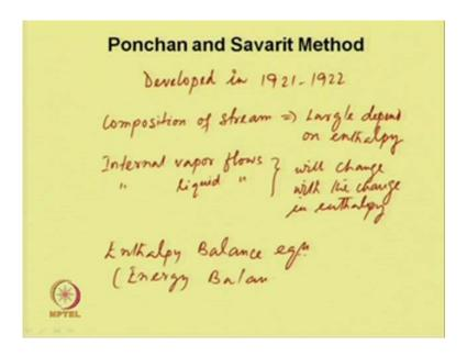
In this case with the total material balance and species mol balance, another balance which is the enthalpy balance is considered, if the composition of stream largely depend on enthalpy. Then the internal liquid and vapor flow from stage to stage will change. Internal vapor flows and internal liquid flows will change, change with the change in enthalpy.
