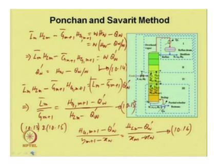
Now, 10.11 this energy balance equations we can write as L m bar H L m minus G m plus 1 bar H G m plus 1 is equal to w H w minus Q w which is equal to w into H w minus Q w by w. From this we can write L m bar H L m minus G m plus 1 bar H G m plus 1 would be equal to W Q w dash where Q w dash is equal to H w minus Q w by w.
