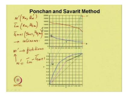
The discussions we have done in case of the rectifying section if we extend the similar discussion over here we could see we have the points over here which is m dash m is the point which is bottoms which coming out and the point m dash which is x w Q w dash and L m bar which is x m H L m and the points G m plus 1 bar which is y m plus 1 and H G m plus 1. So, this three points they are collinear.
