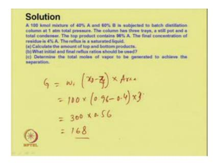
So, we can calculate G which is equals to W i x D minus Z f into area under the curve, so which is equal to 100 multiplied by 0.96 minus 0.4 into is 3 unit. So, it would be equal to 300 multiplied by 0.56 which is equal to 168. So, this way we can determine the total moles of the vapor which is generated to achieve this separation, and the initial and final reflux ratio and the amount of top and bottom products.
