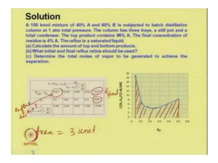
So, the area under the curve for this integral is this, so this is the area is around 3. Now, area is known to us, then the initial reflux which could be used calculate the amount of top and bottom products we have already calculated. What initial and final reflux ratio
