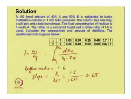
And then the integral equations, we know 1 n W i by W f would be equal to W f to W i x w f to x w i dx w divided by x D minus x w. And the reflux ratio is given 1.6, therefore slope would be equal to R by R plus 1 which is equal to 1.6 divided by 1.6 plus 1 which is equal to 0.615.
