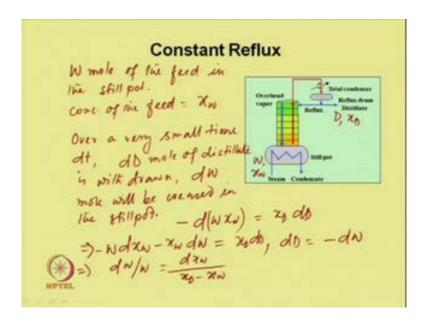
Now let us consider the first case which is constant reflux operation. We will discuss constant reflux operations. We have taken say W mole of the feed in the still pot, and its concentration of the feed is x w. Assume very small time free out over a very small time delta t – dt, dD is the distillate and this is the W and its x D and its composition is x w.
