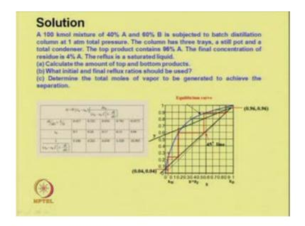
Let us see the table. The first one has slope of 0.417 x w is 0.5, so we could able to calculate this one. Similarly, for the second we have operated 0.521. So, we have a set of data with these we can plot this 1 by x D minus x w square into 1 minus d l by d g verses x w. So, we can calculate the area under the curve for this integral.
