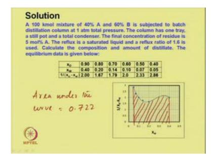
So, which is plotted over here and the area between this, so area under this curve, this is by any method we can obtain the area 0.722. So, area under the curve we can obtain.
