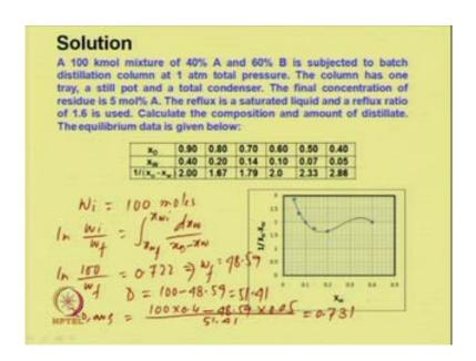
And then we know the initial amount of moles taken. So, W i which is 100 mole and we know l n W i by W f is equal to integral x w f x w i d x w by x D minus x W. So, here we
