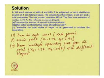
Now, draw the equilibrium line the data is given. Second will locate point x D which is 0.96. From this since the x D is constant the slop of the particular line will change. So, we will draw from starting from this point, we will draw different operating lines, draw multiple operating line from the point x D is equal to 0.96 x D is equal to 0.96.
